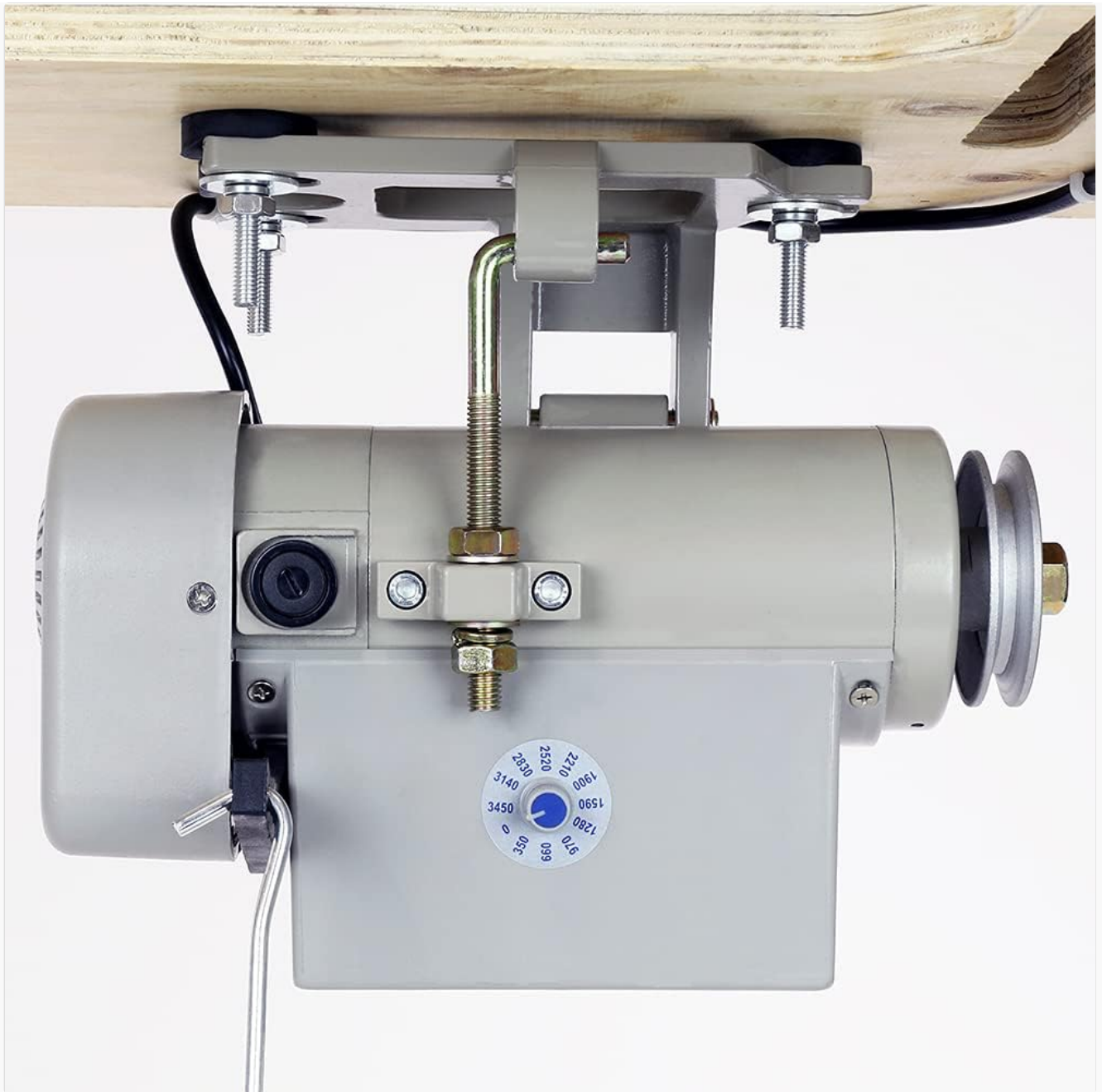
Figure 4.2: Close-up of the servo motor mounted beneath the machine table.
