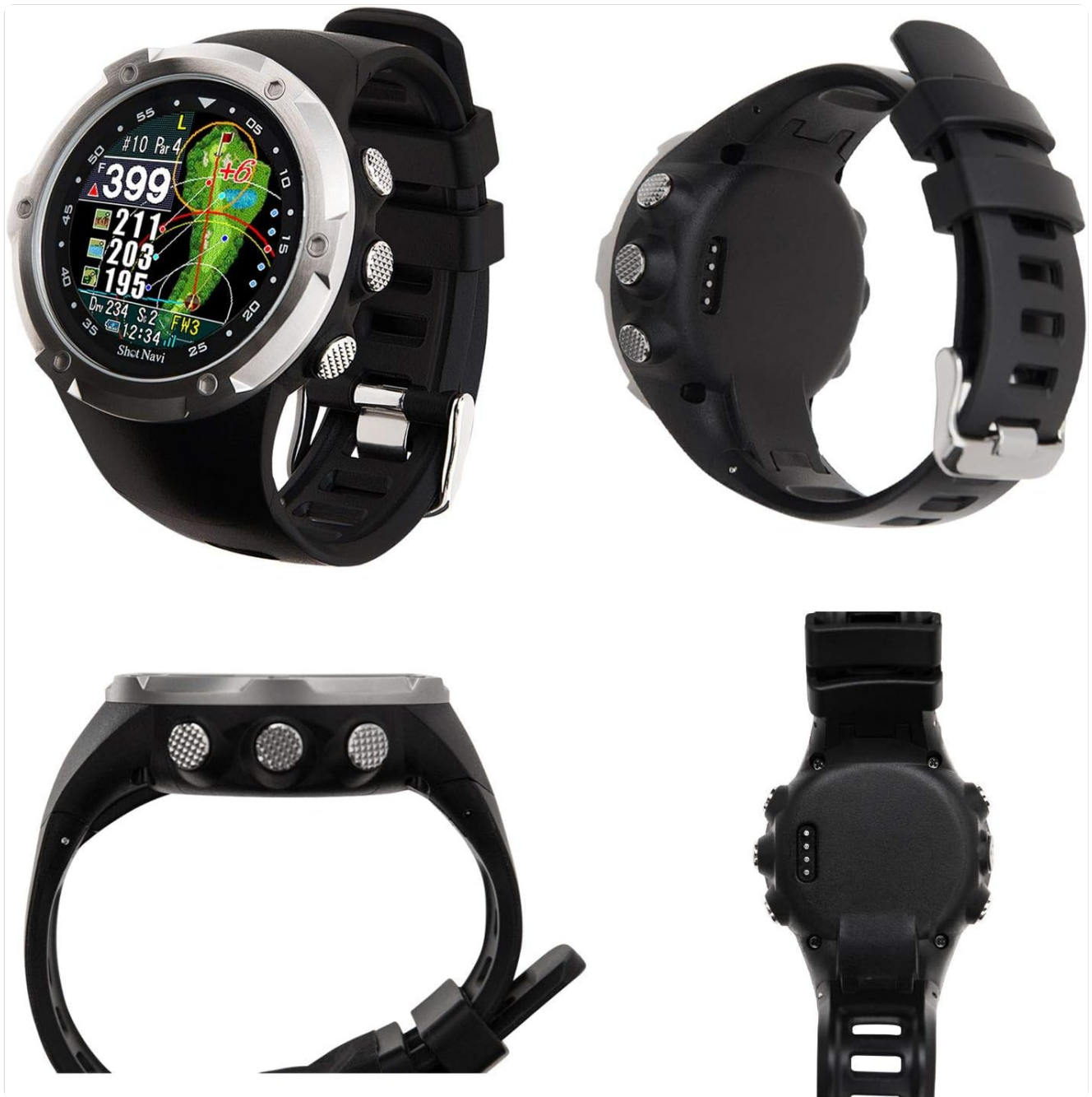
Various views of the Shot Navi W1 Evolve, illustrating its design, button placement, and charging contacts on the rear.
