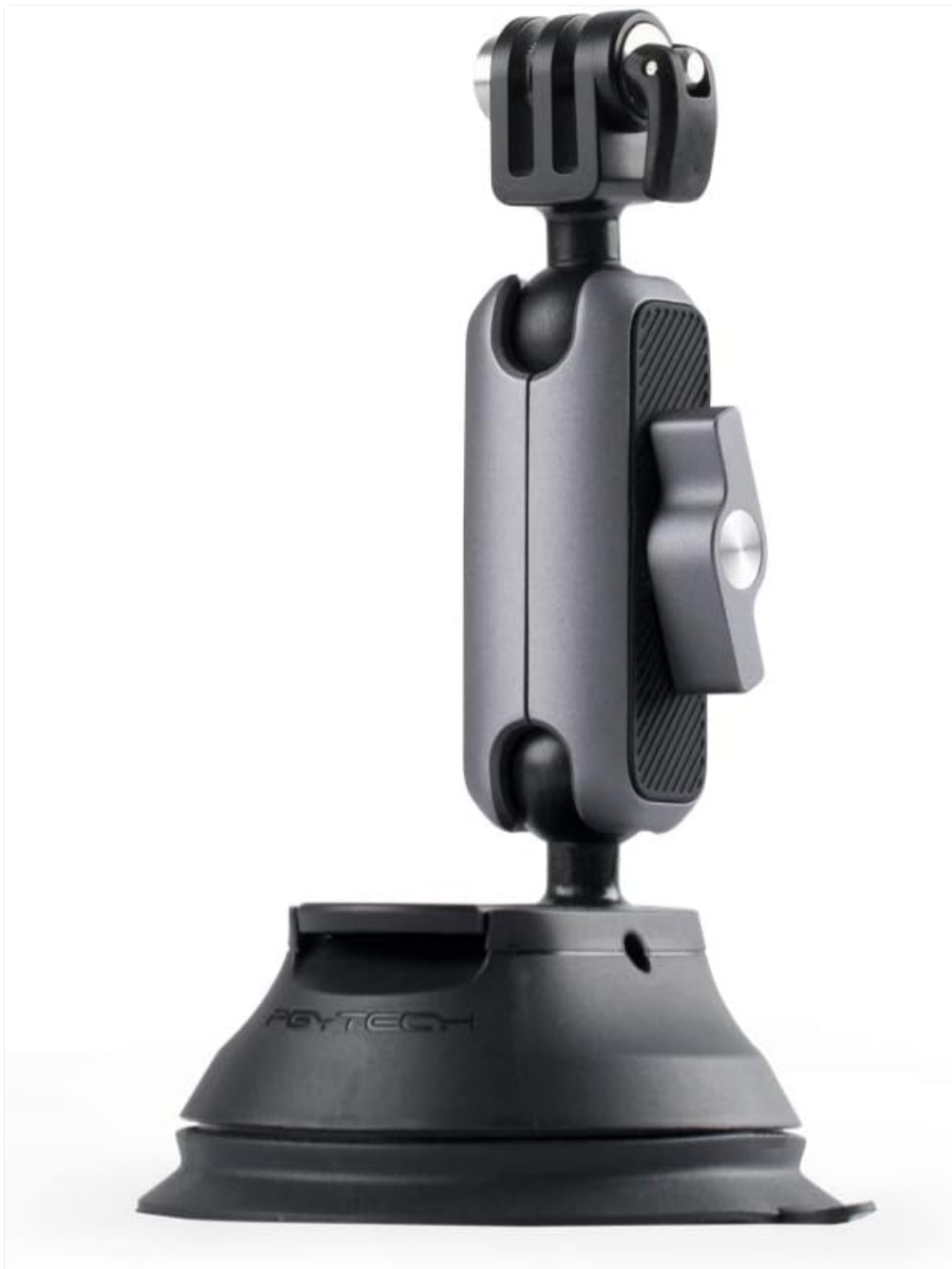
Figure 3: Side view of the mount, illustrating the double ball joint for angle adjustments. The central knob is used to loosen and tighten the joints.
