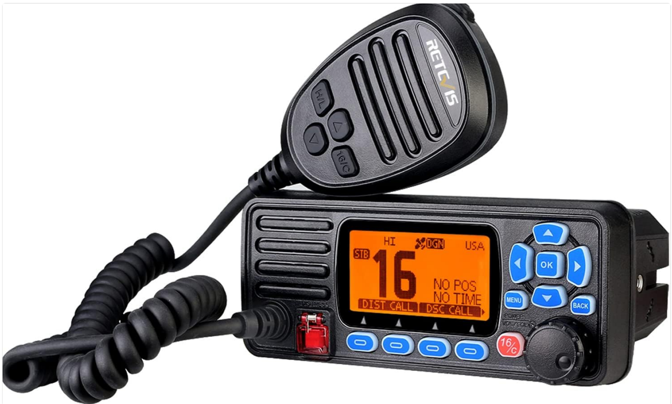
Figure 1: Retevis RA27 Fixed Mount Marine Radio with Handheld Microphone.
