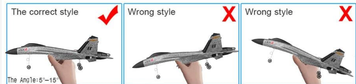
Image 4.2: Visual guide for ground take-off and handthrow take-off techniques, including correct and incorrect handthrow angles.
