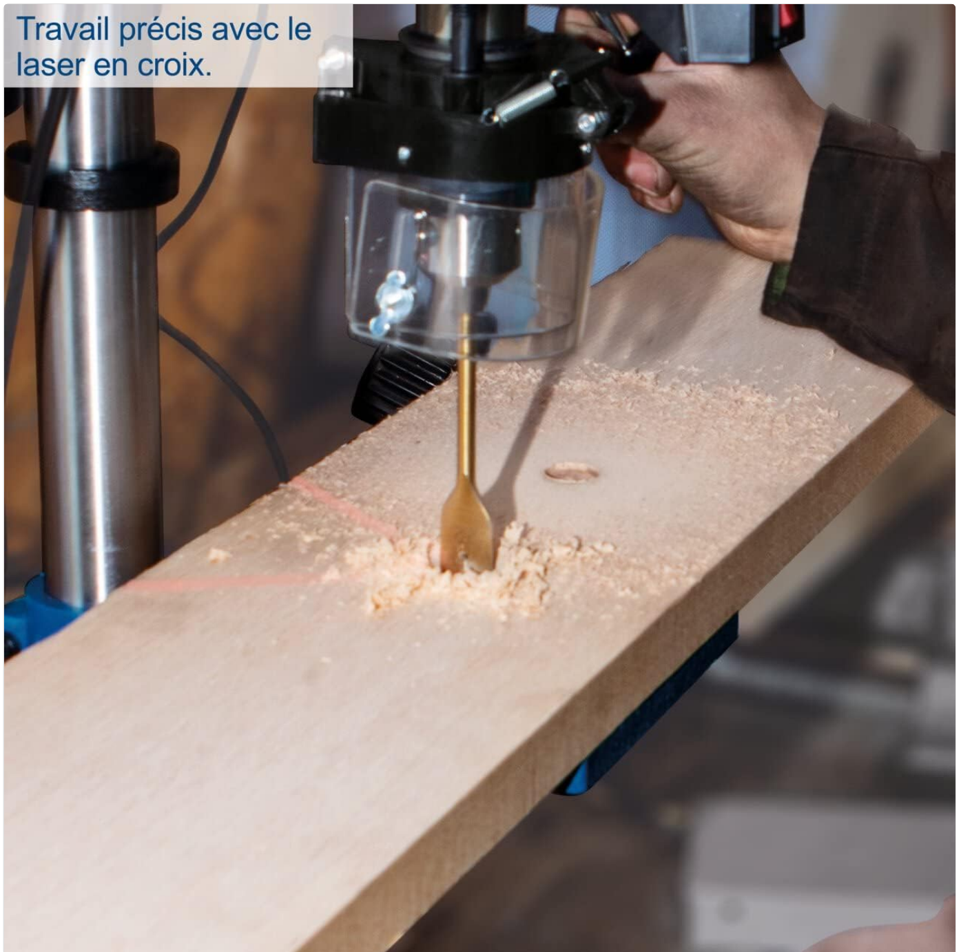
Figure 9: Achieve precise drilling results with the integrated cross laser, ensuring accurate hole placement on various materials.
