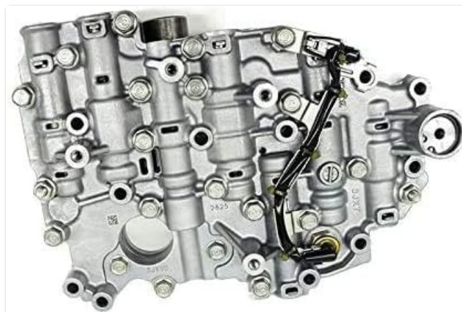
Figure 4.2: Bottom view of the valve body, illustrating hydraulic channels and mounting points.
