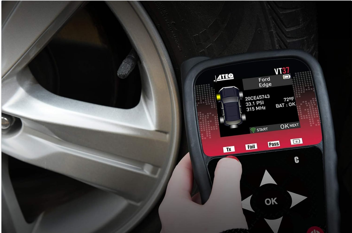
Image Description: ATEQ VT37 tool held against a car tire, displaying sensor data on its screen, indicating successful reading.
