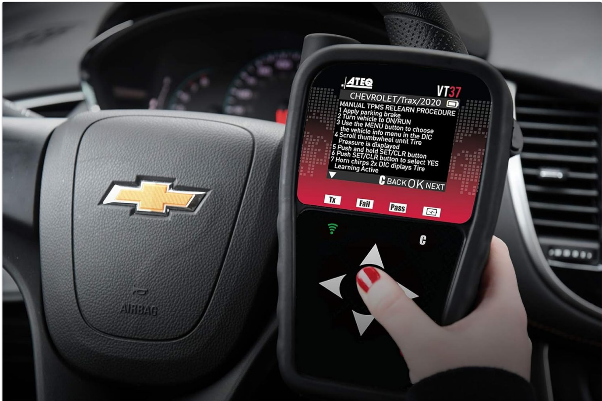
Image Description: The ATEQ VT37 tool screen showing detailed steps for a manual TPMS relearn procedure for a Chevrolet/Trax vehicle, held inside the car's cabin.
