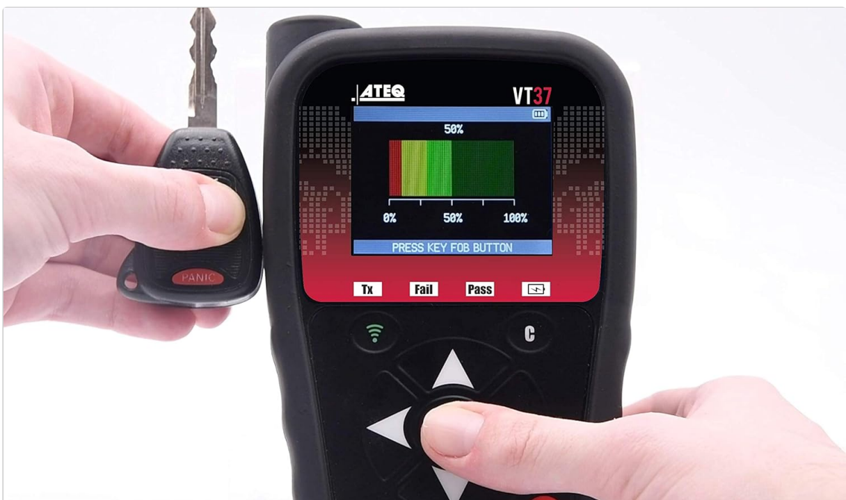
Image Description: A user holding a car key fob next to the ATEQ VT37 tool, which shows a graphical representation of the key fob's signal strength on its display.
