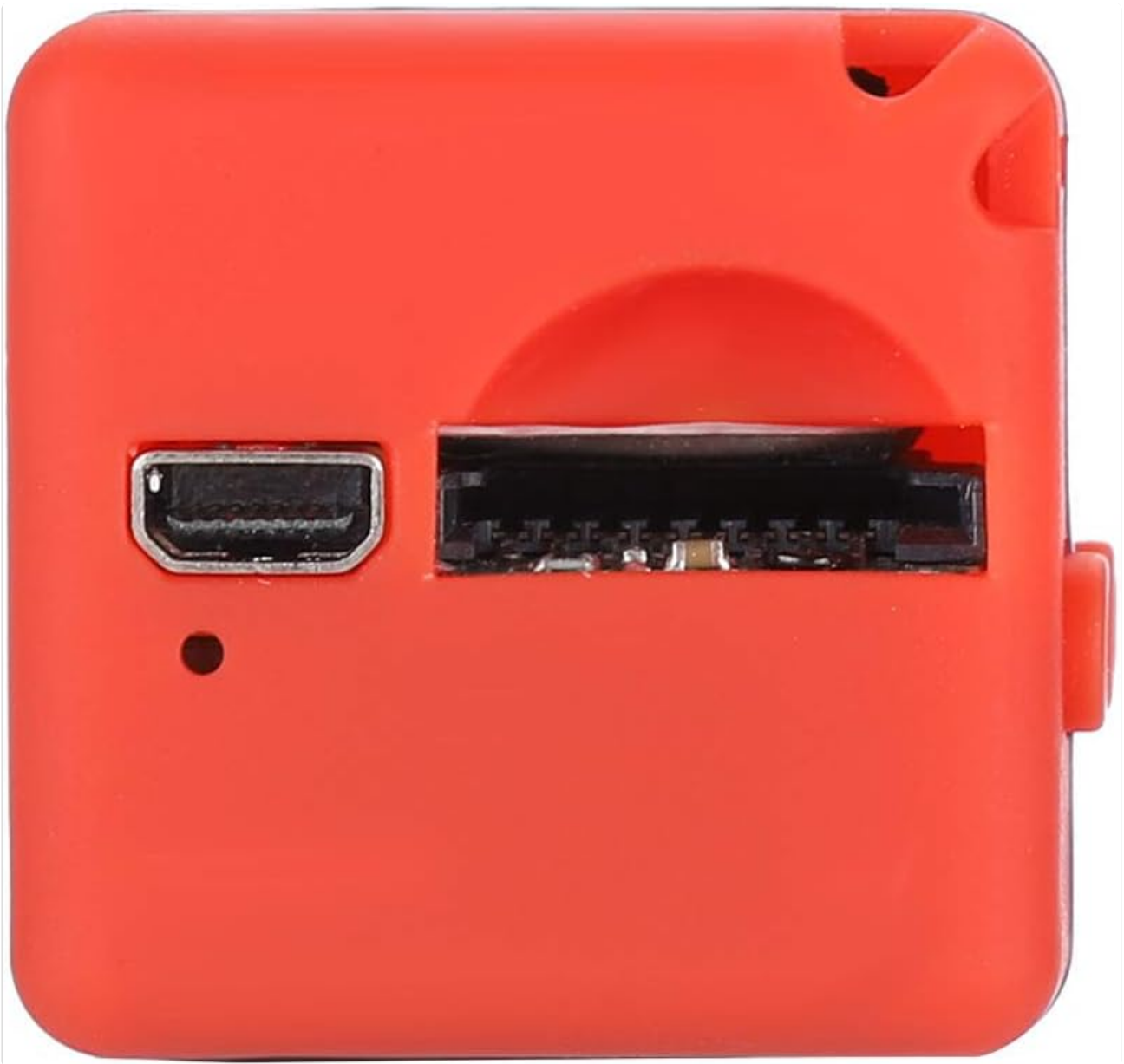
Figure 4.1: Side view of the camera, indicating the Micro SD card slot and Mini USB port.
