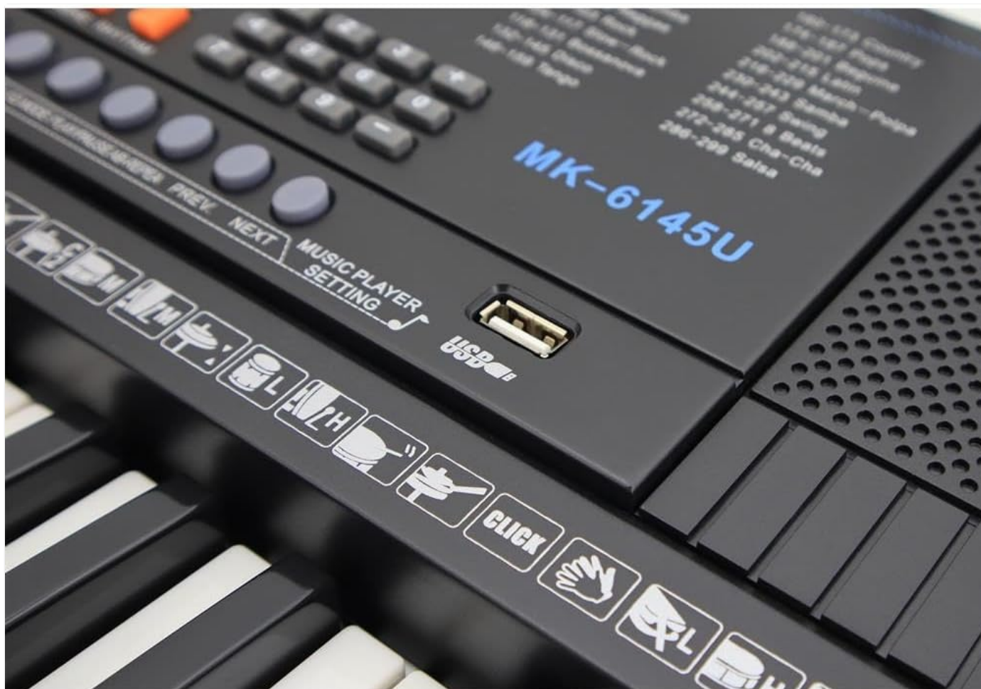
Figure 4.3: Close-up of the control panel on the JWIN MK-6145U, detailing the LCD screen, function buttons, and the USB port for music playback.
