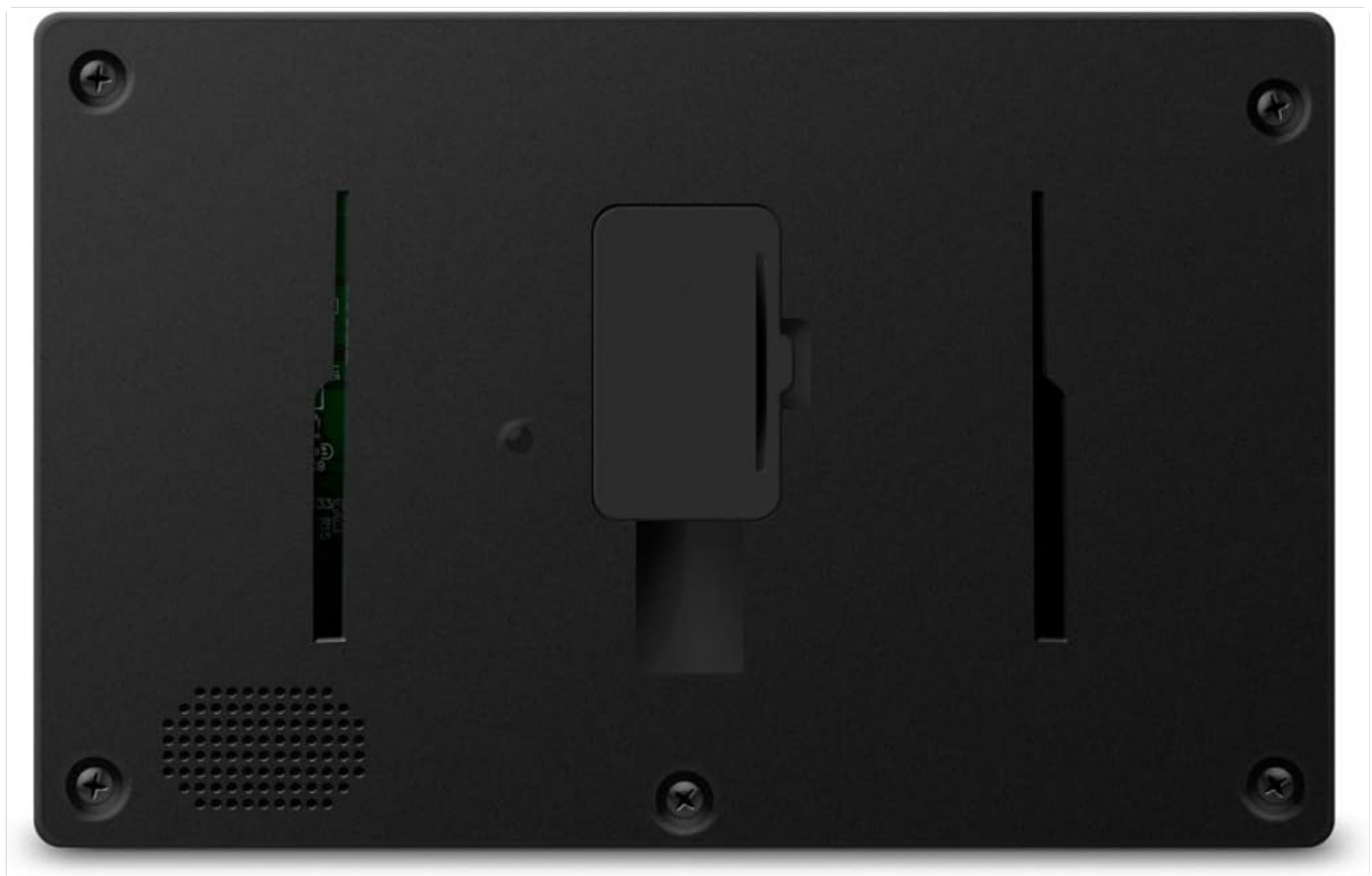
Figure 4.2: The rear view of the indoor display unit, illustrating the cable connection port, TF card slot, and mounting points for attachment to the door bracket.
