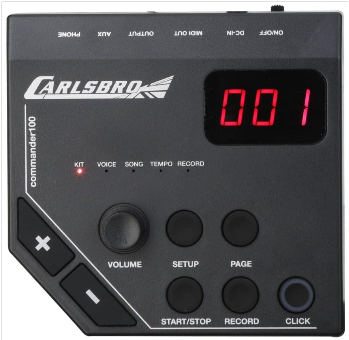
Figure 3.3: The Commander Module 101, showing controls and connection ports.
