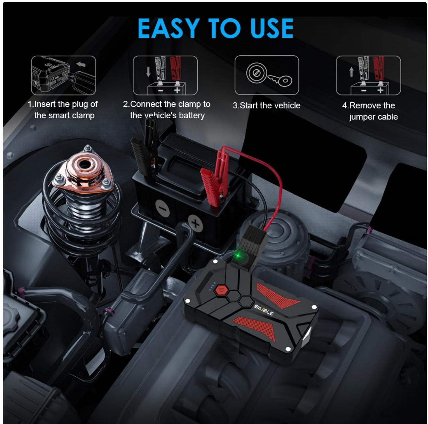
Figure 4: Visual guide for the jump-starting process, from connecting the cable to starting the vehicle.
