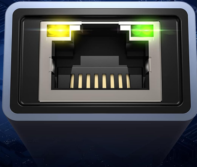
Image 4.1: A close-up view of the adapter's RJ45 port showing the Signal (yellow) and Connection (green) LED indicators.
