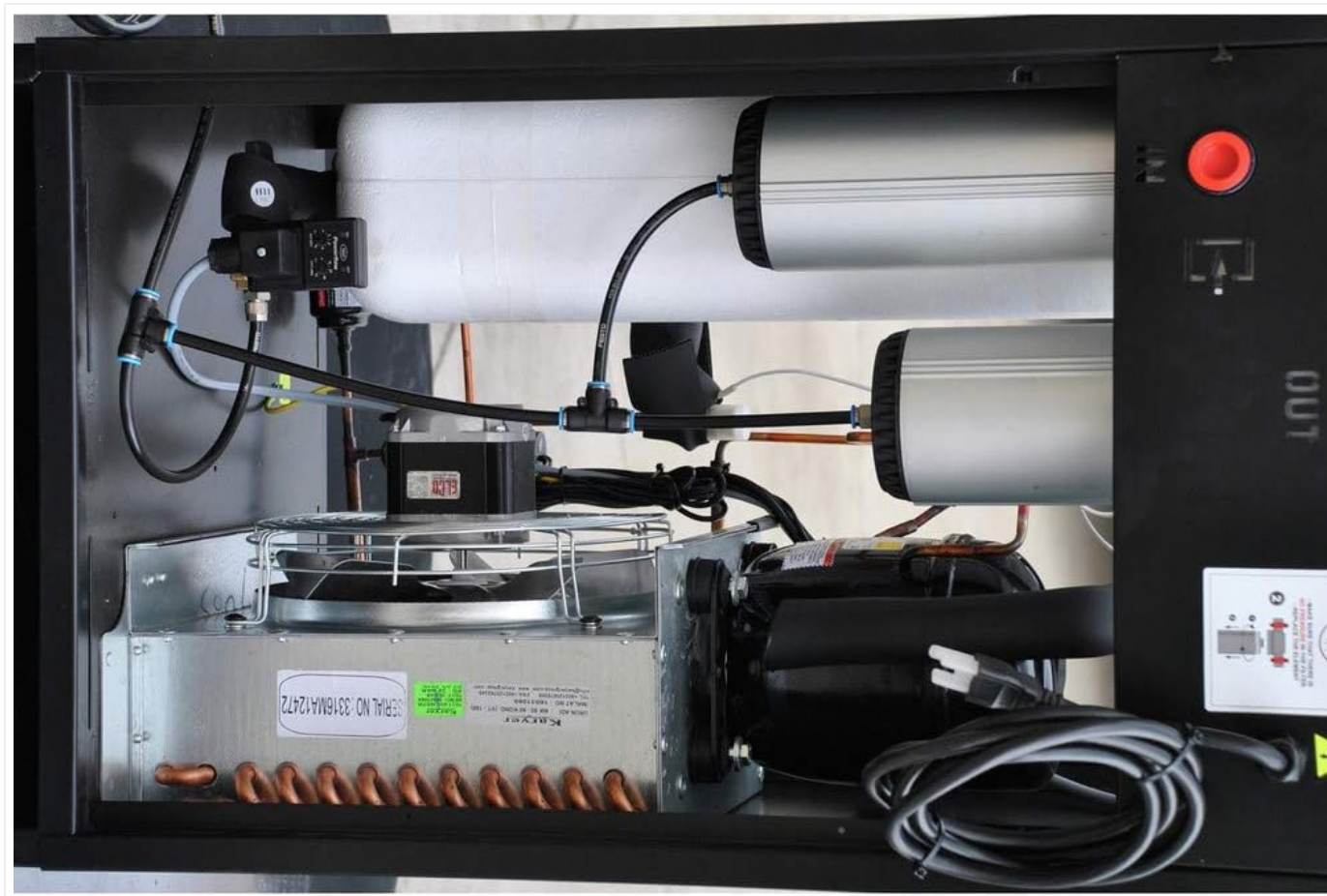
Figure 6: Internal components of the refrigerated air dryer, including filters.
