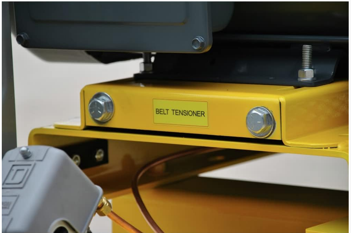
Figure 3: The belt tensioner mechanism, designed for easy adjustment.
