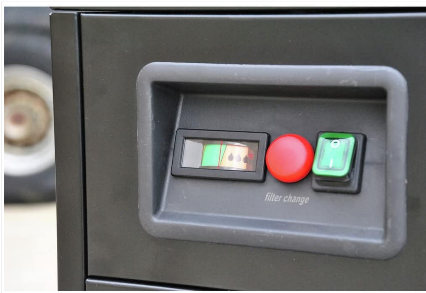
Figure 5: Air dryer control panel with filter change indicator.
