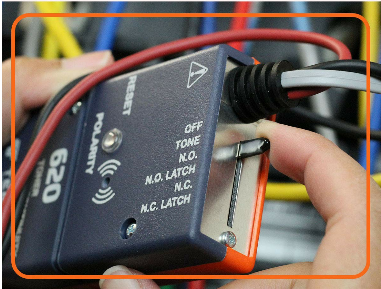
Figure 4: The 6-position slide switch on the tone generator, used to select between OFF, TONE, N.O., N.O. LATCH, N.C., and N.C. LATCH modes.
