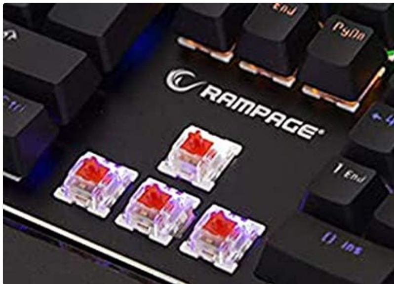
Figure 3.4: Close-up view of the Red mechanical switches, known for their linear feel and quick response.
