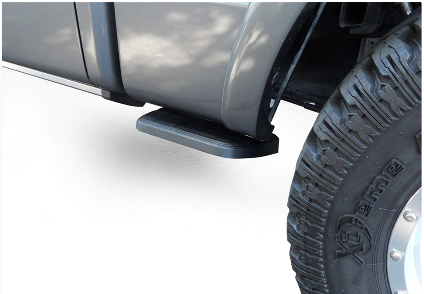
Image: The AMP Research BedStep2 in its retracted position, stowed neatly beneath the truck's body.
