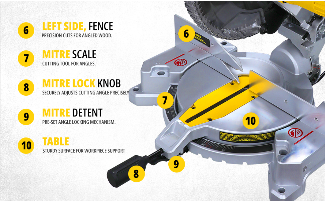
Figure 2: Upper Components of the Mitre Saw
