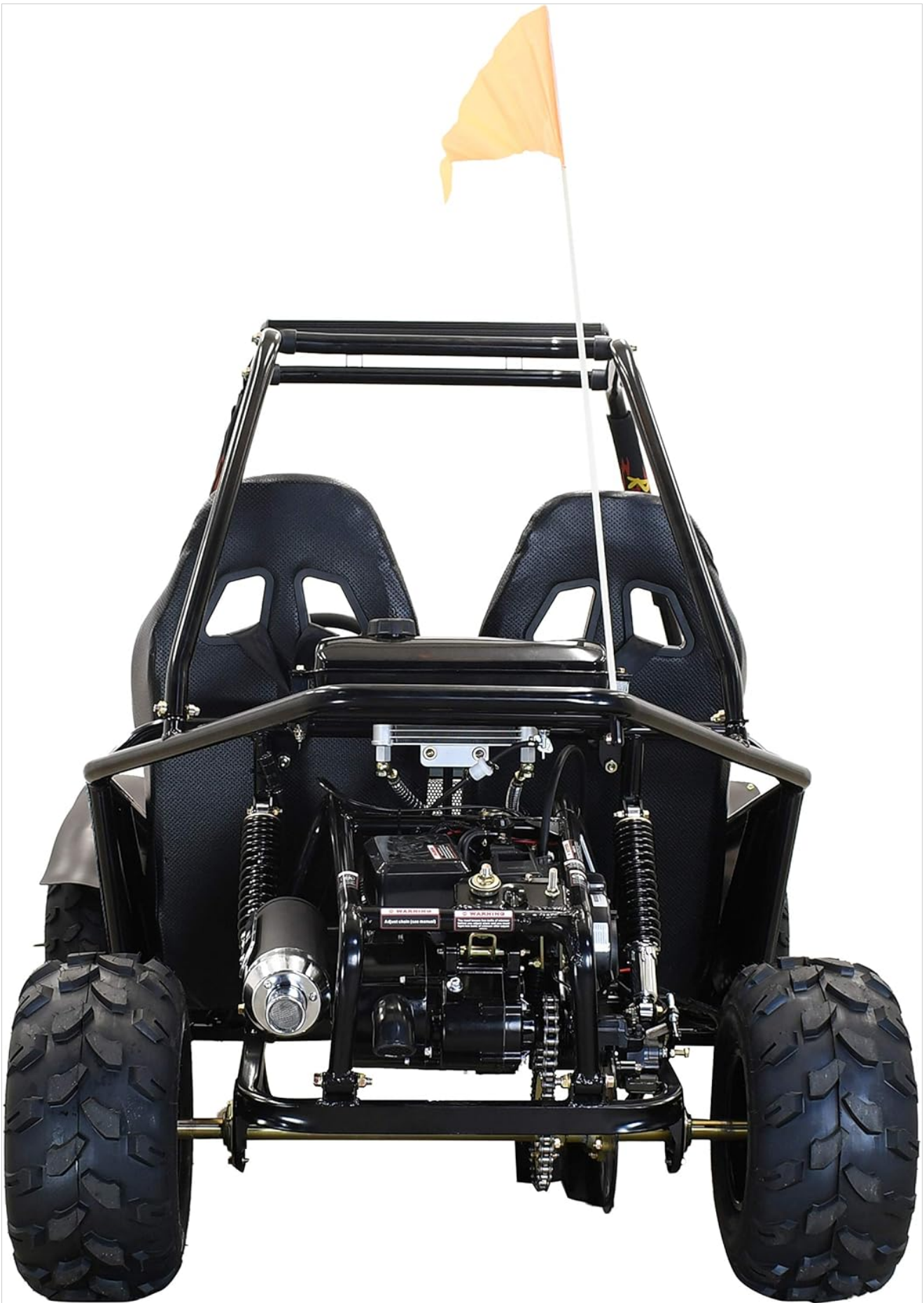
Figure 4.1: Rear view of the Massimo GKM 200 Go-Kart, showing the engine compartment and rear suspension.
