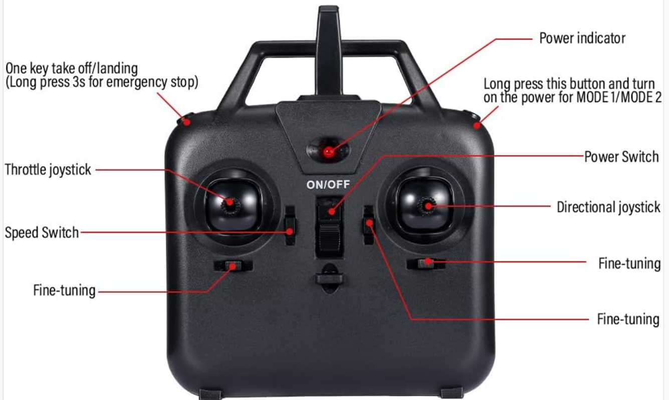
Image 4.5: Diagram illustrating the remote controller's layout, including the power indicator, power switch, throttle joystick, directional joystick, speed switch, fine-tuning buttons, and one-key take off/landing/emergency stop button.
