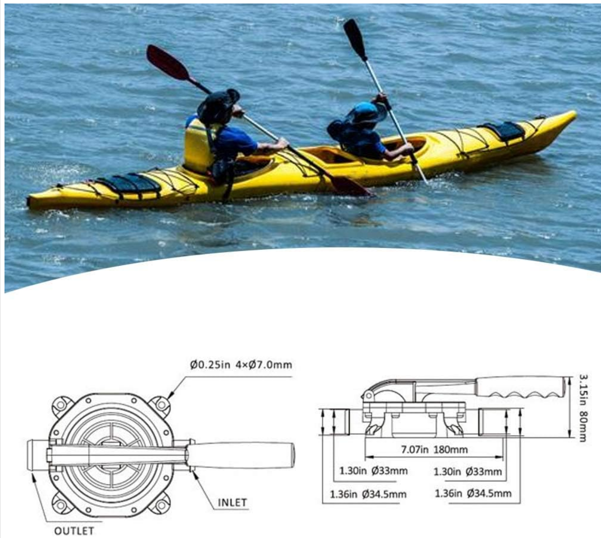
Figure 4.1: Technical diagram illustrating the pump's dimensions, including inlet and outlet hose diameters, and overall body size.
