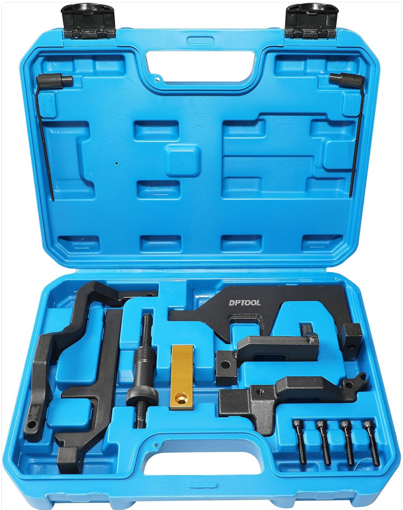
Image 1.1: The complete DPTOOL Camshaft Alignment Timing Tool Set stored in its protective blue case.
