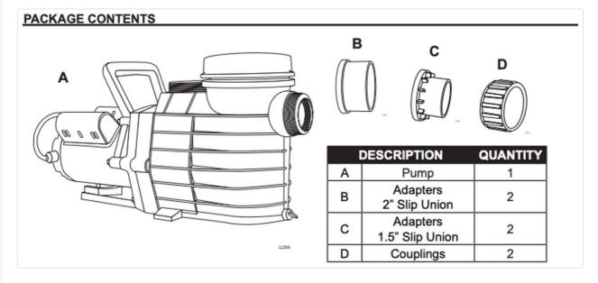
Image: Package Contents Diagram. This illustration details the main pump unit (A) and the included connection accessories: 2-inch slip union adapters (B), 1.5-inch slip union adapters (C), and couplings (D).
