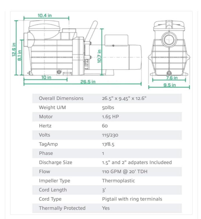
**Image:** Product Dimensions and Specifications. This image provides a detailed technical drawing with key dimensions of the pump and a table summarizing its electrical and performance characteristics.
