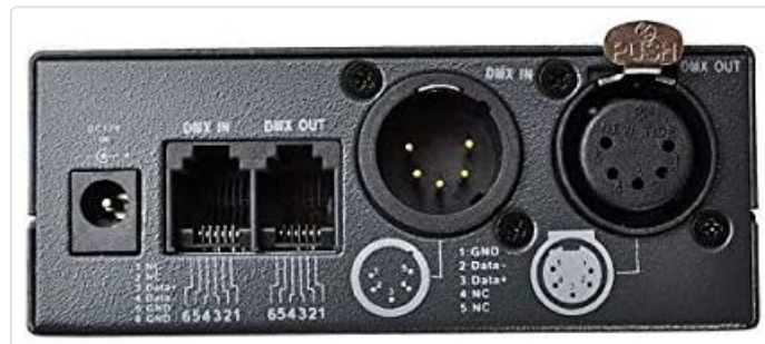
Figure 3.2: Rear View of the LITEPUTER CX1C DMX Tester. This image displays the rear panel, highlighting the DC 12V power input, DMX IN and DMX OUT ports (both RJ45 and 5-pin XLR connectors), and pinout diagrams.
