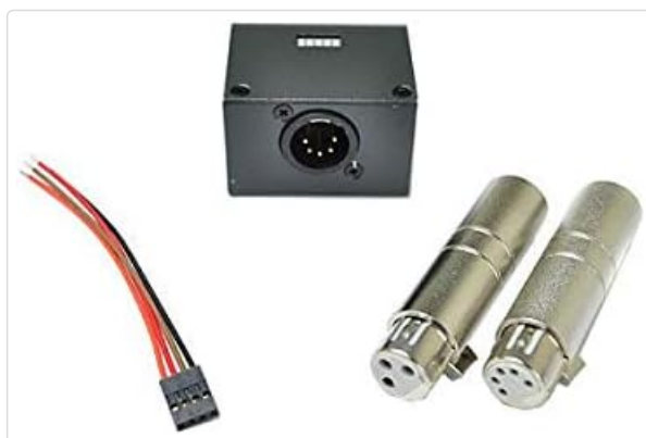
Figure 3.3: LITEPUTER CX1C DMX Tester Accessories. This image shows typical accessories that may be included with the DMX tester, such as a power cable and XLR adapters, facilitating various connection types.
