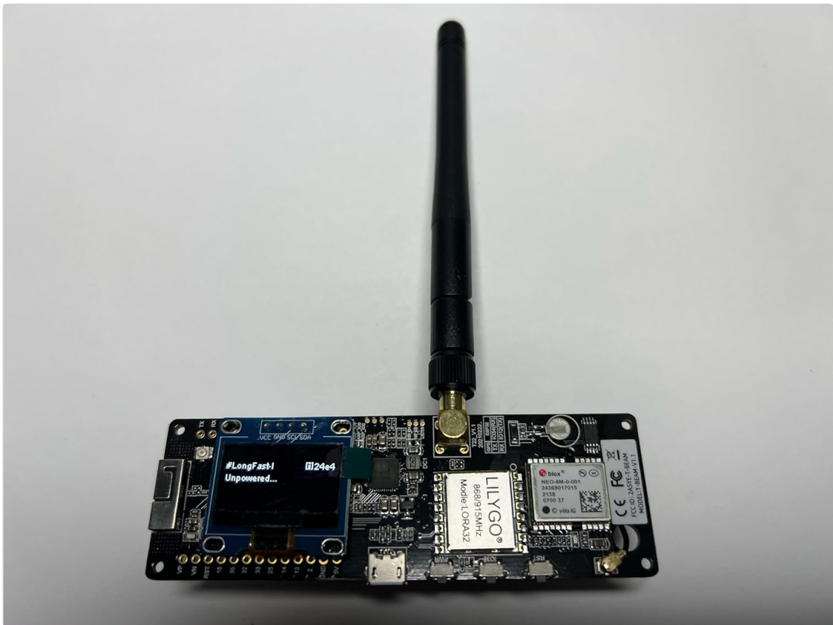
Figure 1: TTGO Meshtastic T-Beam V1.1 board. The image shows the main board with the LoRa antenna connected, the OLED display showing "Unpowered...", and various components including the ESP32, LoRa module, and GPS module.
