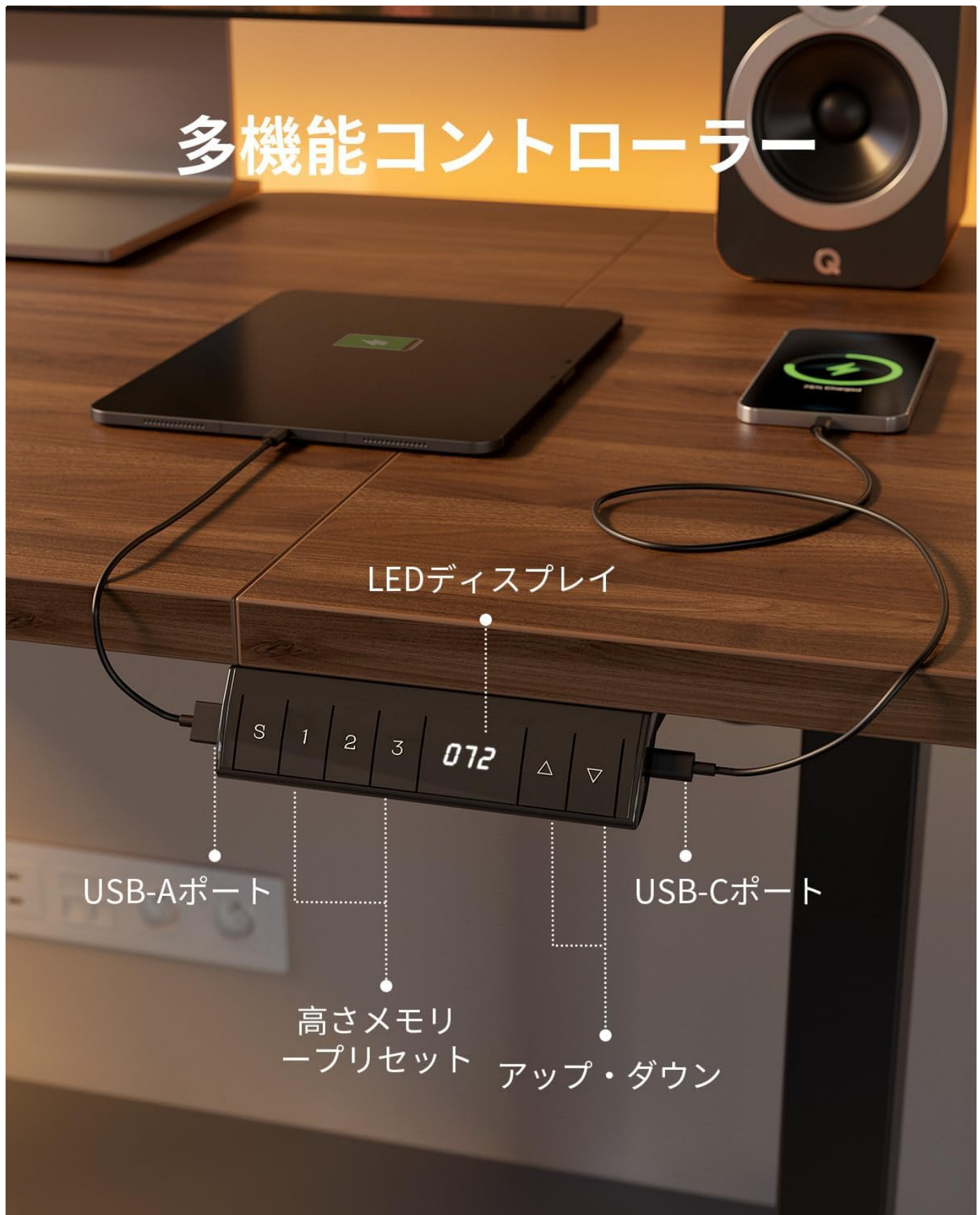
Figure 2: Multi-functional control panel with USB ports.
