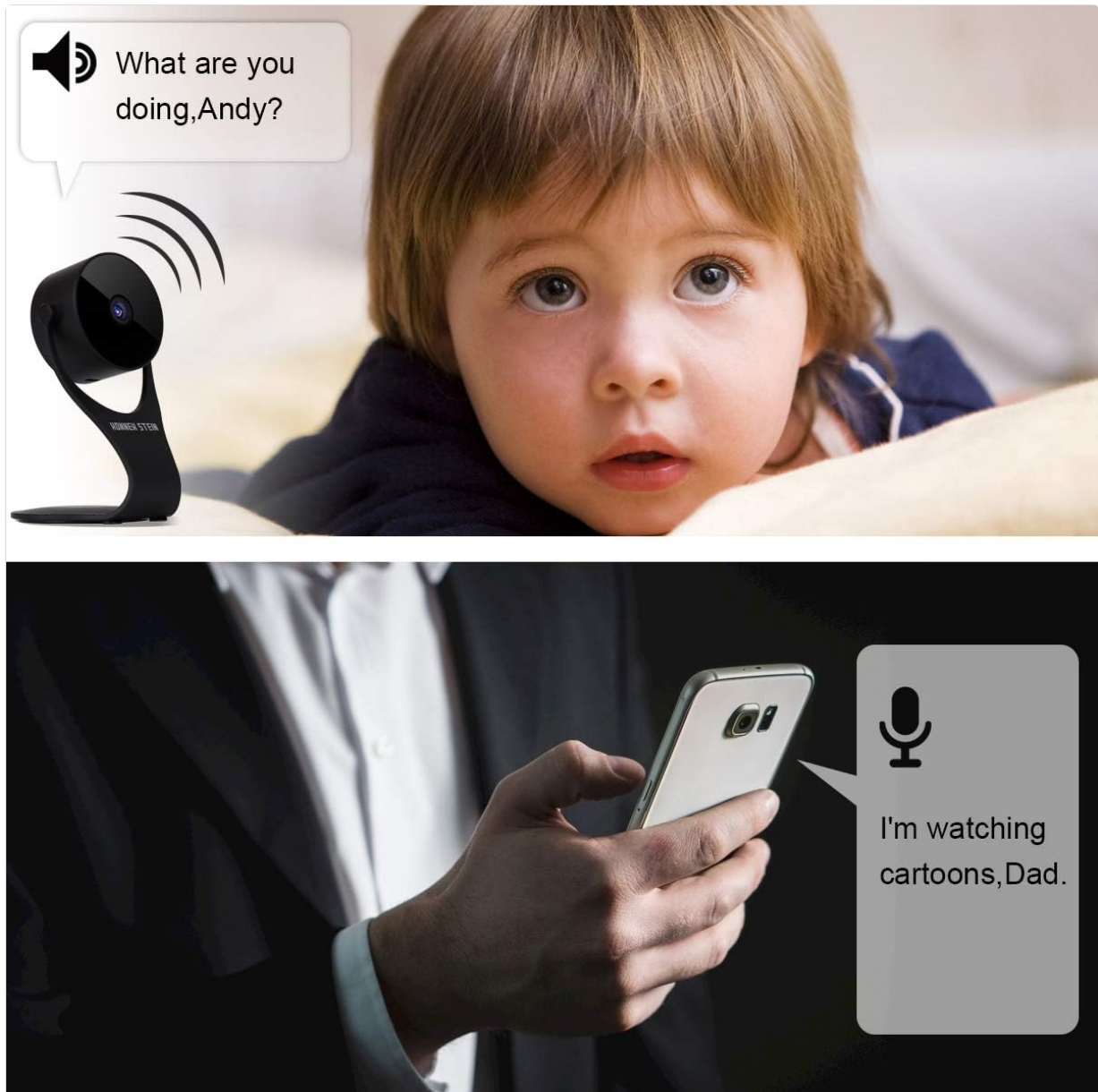
Figure 4.2.1: Illustration of the two-way audio feature, enabling communication between the user and the camera's environment.
