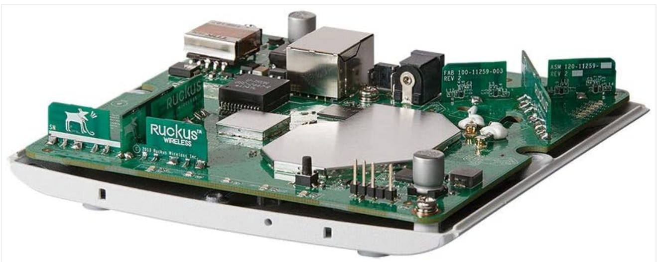
Figure 4: Internal view of the Ruckus R320 Access Point, showing the circuit board and components.
