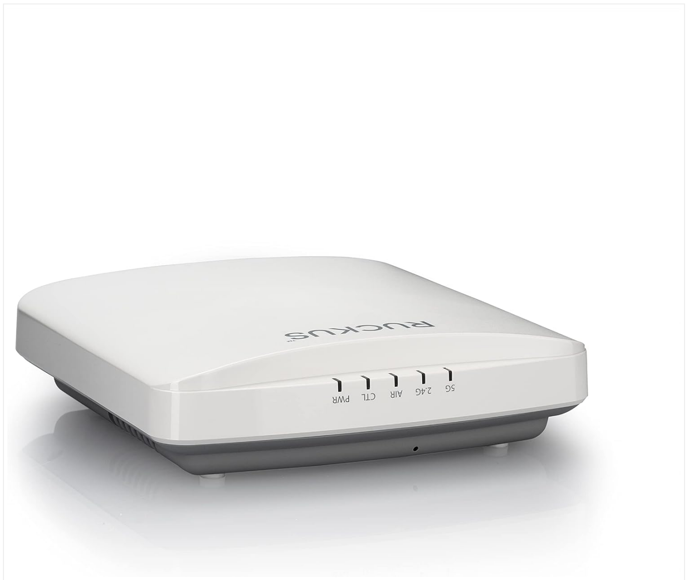
Figure 4: Top view of the Ruckus R550, highlighting the status LED indicators.
