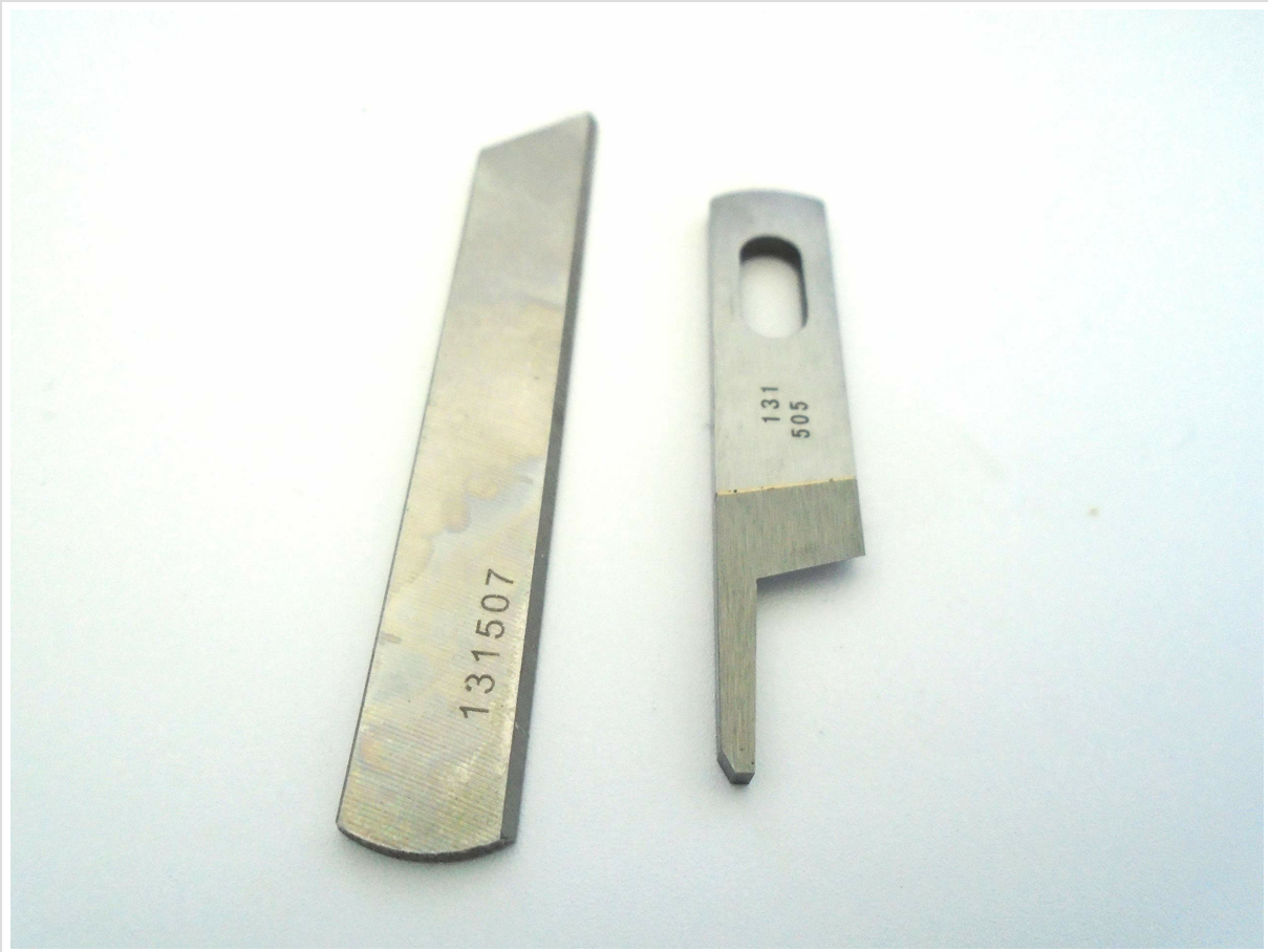
Image 1: The NGOSEW Upper Knife (131-50503) and Lower Knife (131-50701) set. The upper knife is typically the moving blade, and the lower knife is the stationary blade, working together to cut fabric edges.
