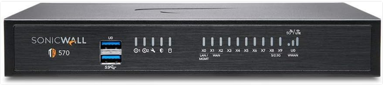
Figure 1: Front view of the SonicWall TZ570 Network Security Appliance. This image displays the compact form factor of the device, featuring USB 3.0 ports and various LED indicators on the front panel.
