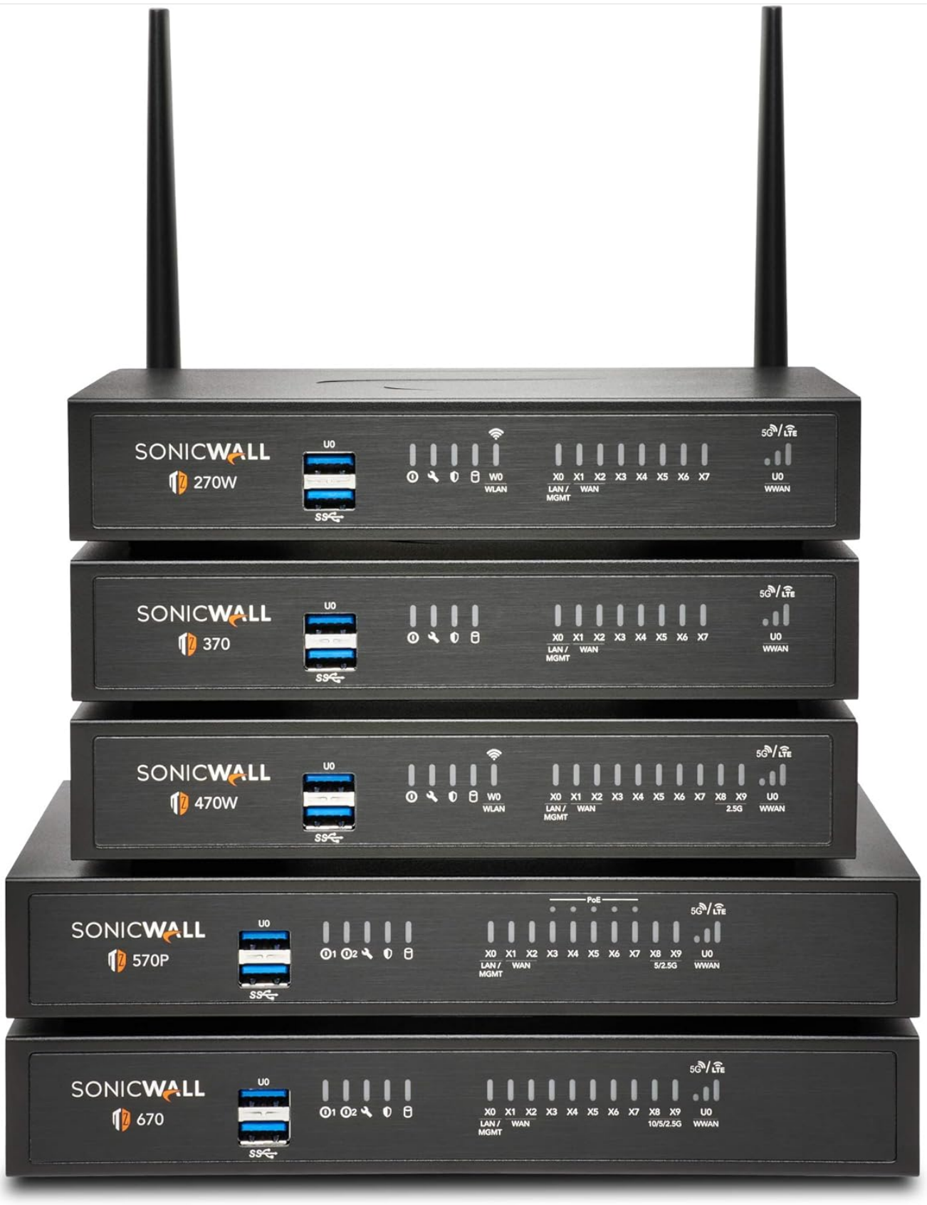
Figure 2: A stack of various SonicWall TZ series firewalls, showcasing the range of appliances available. The TZ570 is part of this series, designed for scalable network security solutions.
