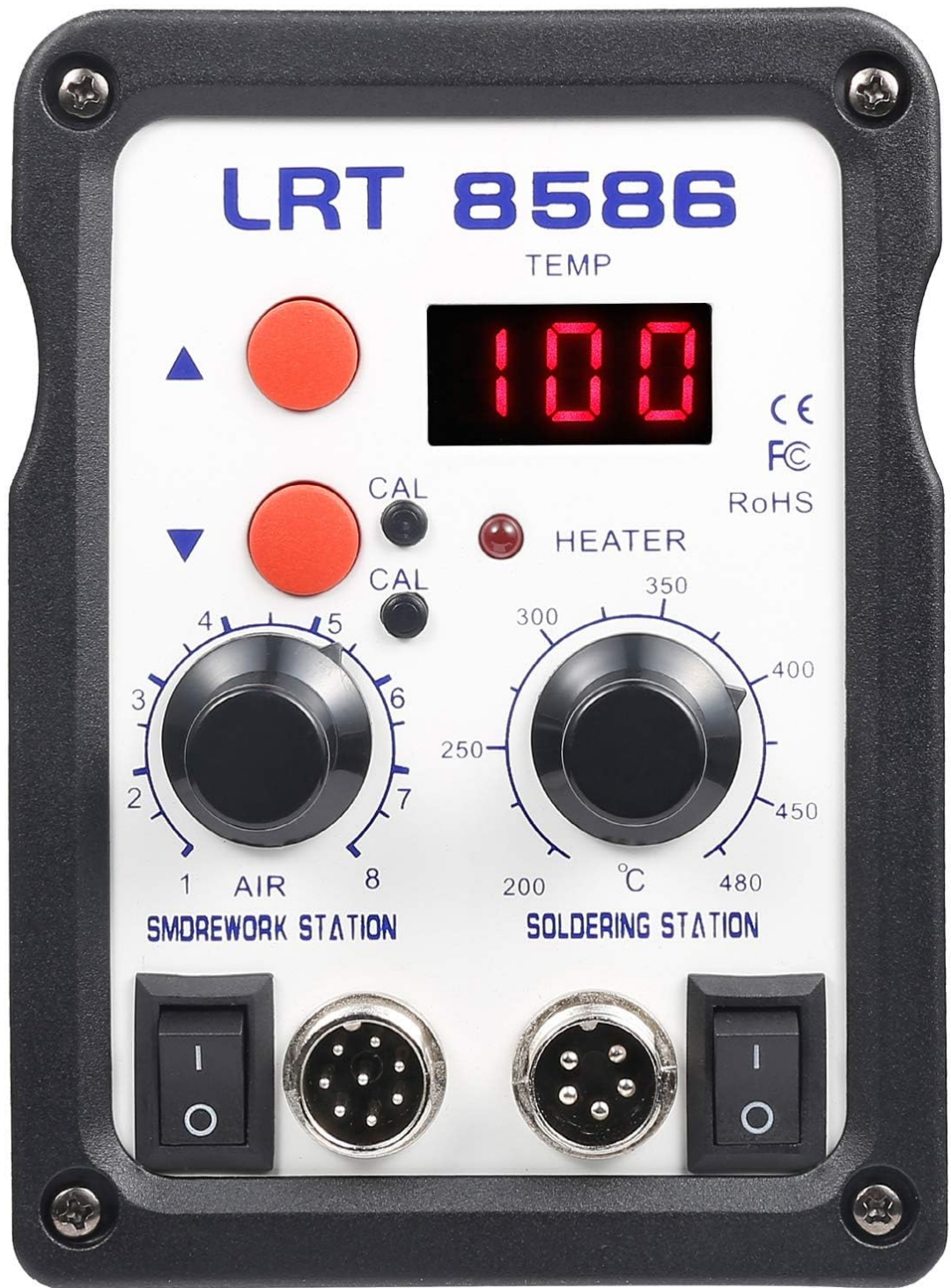
Figure 5.1: Front control panel of the LRT 8586 station.
