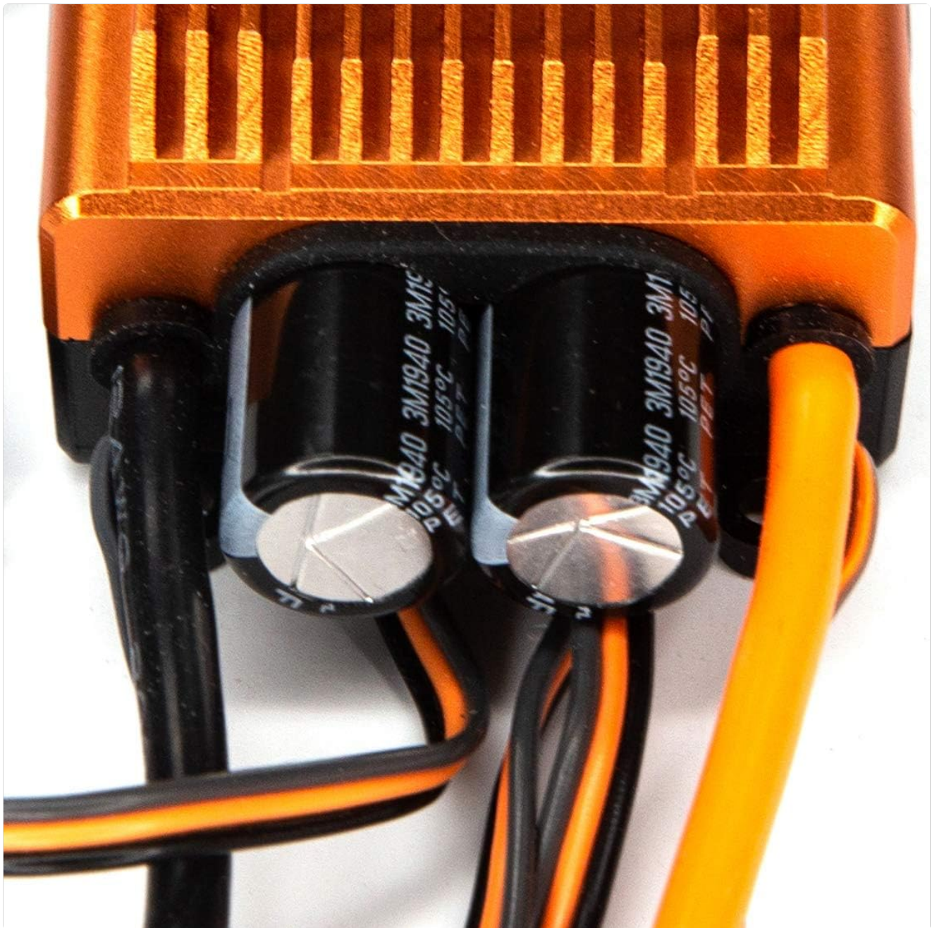
Figure 7.1: Capacitors on the ESC, which should be regularly inspected for any signs of damage or swelling.
