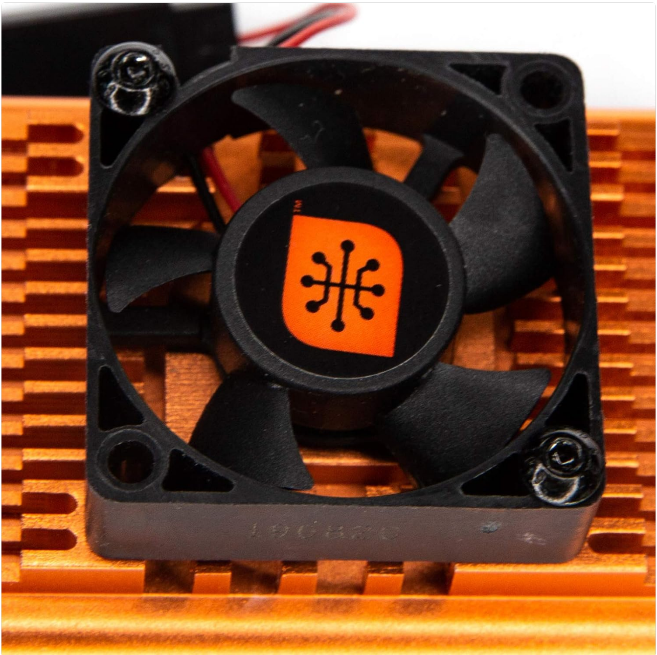
Figure 7.2: The cooling fan, which should be kept clear of obstructions for effective heat dissipation.
