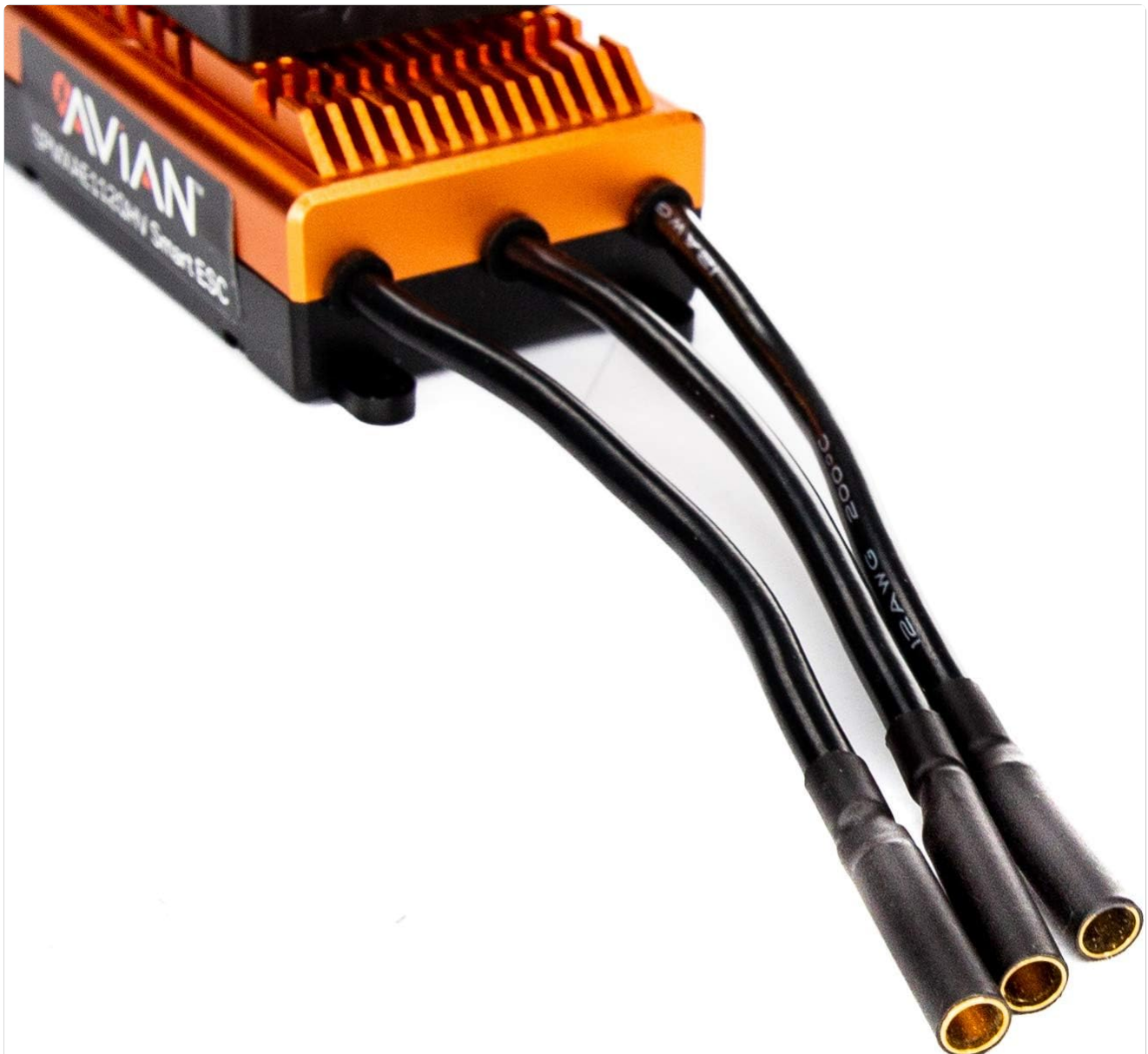
Figure 4.1: Side view of the ESC, illustrating the main power input and motor output connections.
