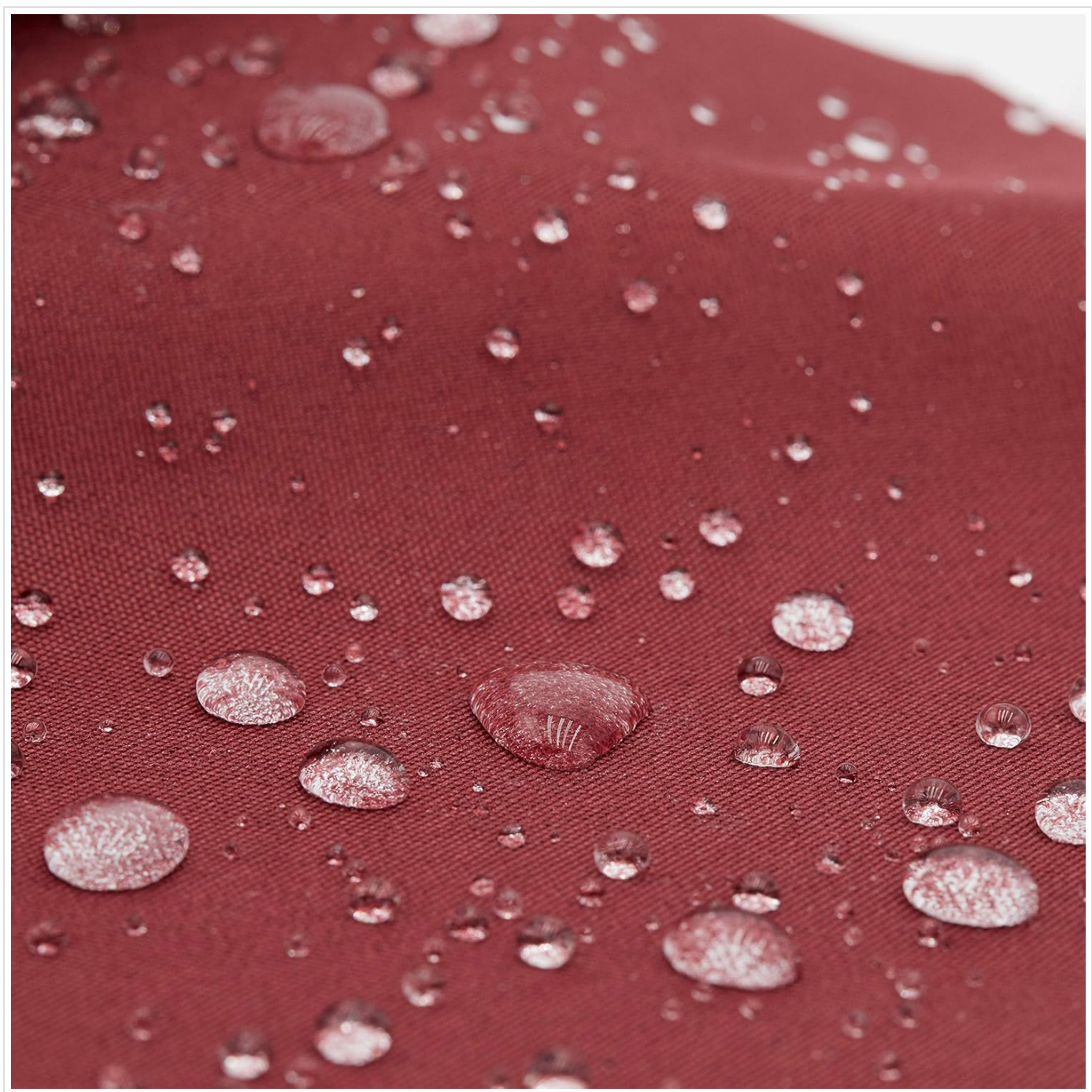
Image: Water beading on the PES 700 PVC-coated polyester roof tarp, illustrating its water-resistant properties.
