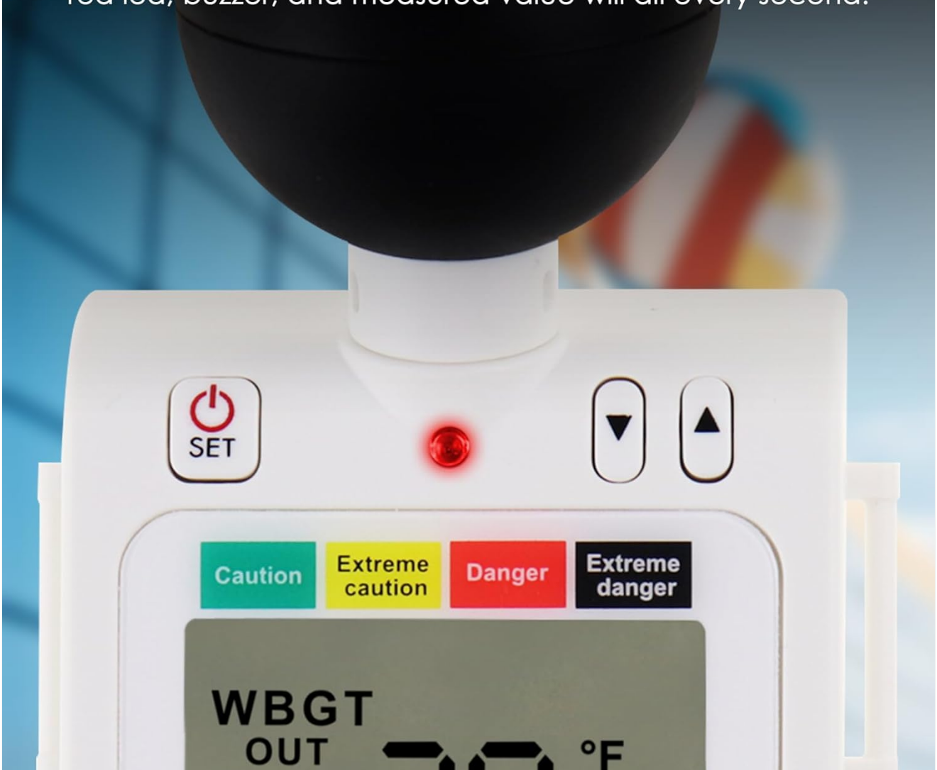
Image 6: The red LED alarm light indicates when measured heat stress values exceed the set threshold.
