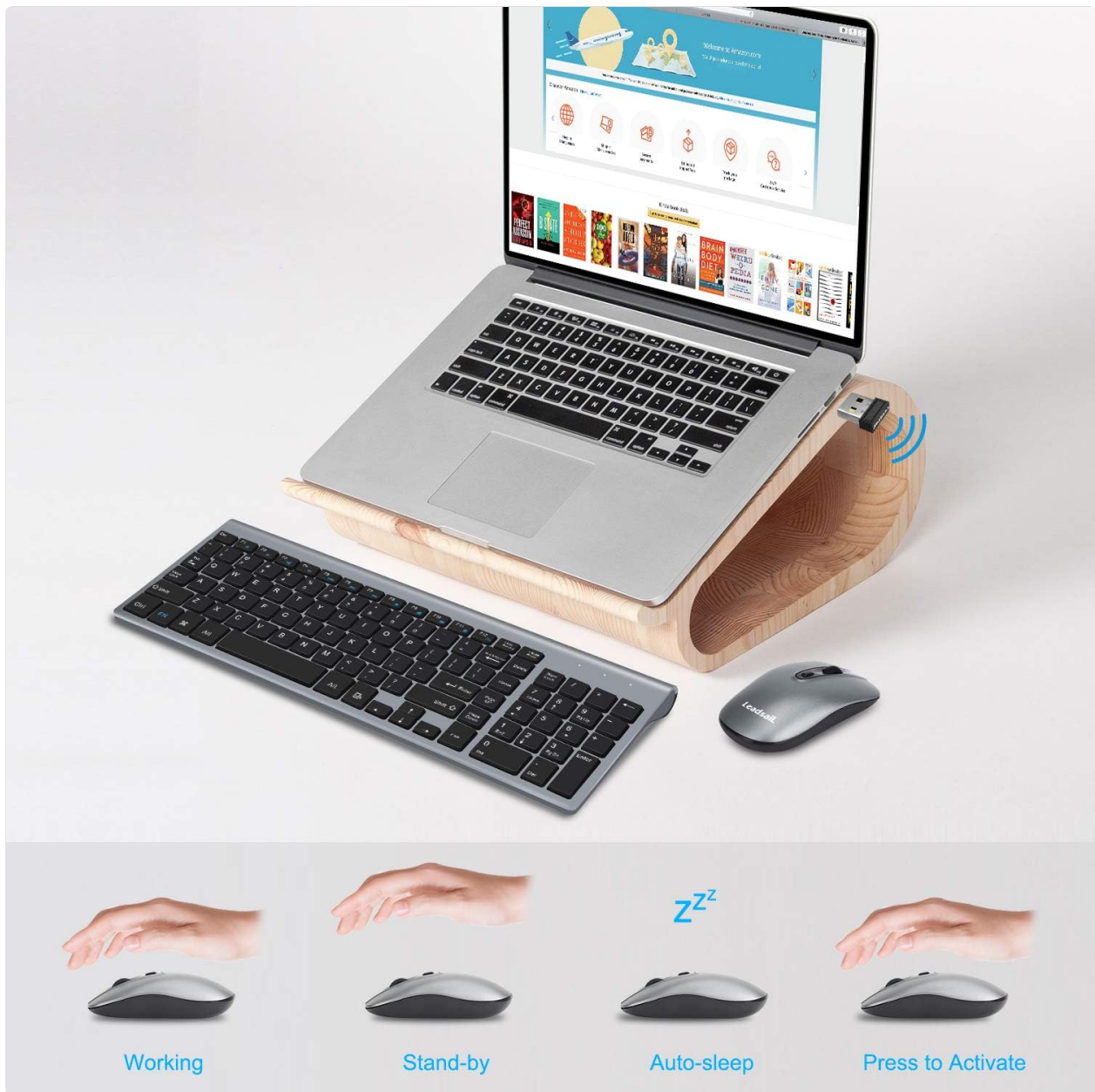
Image 5.1: Visual representation of the mouse transitioning from working to stand-by and auto-sleep modes, and how to activate it.
