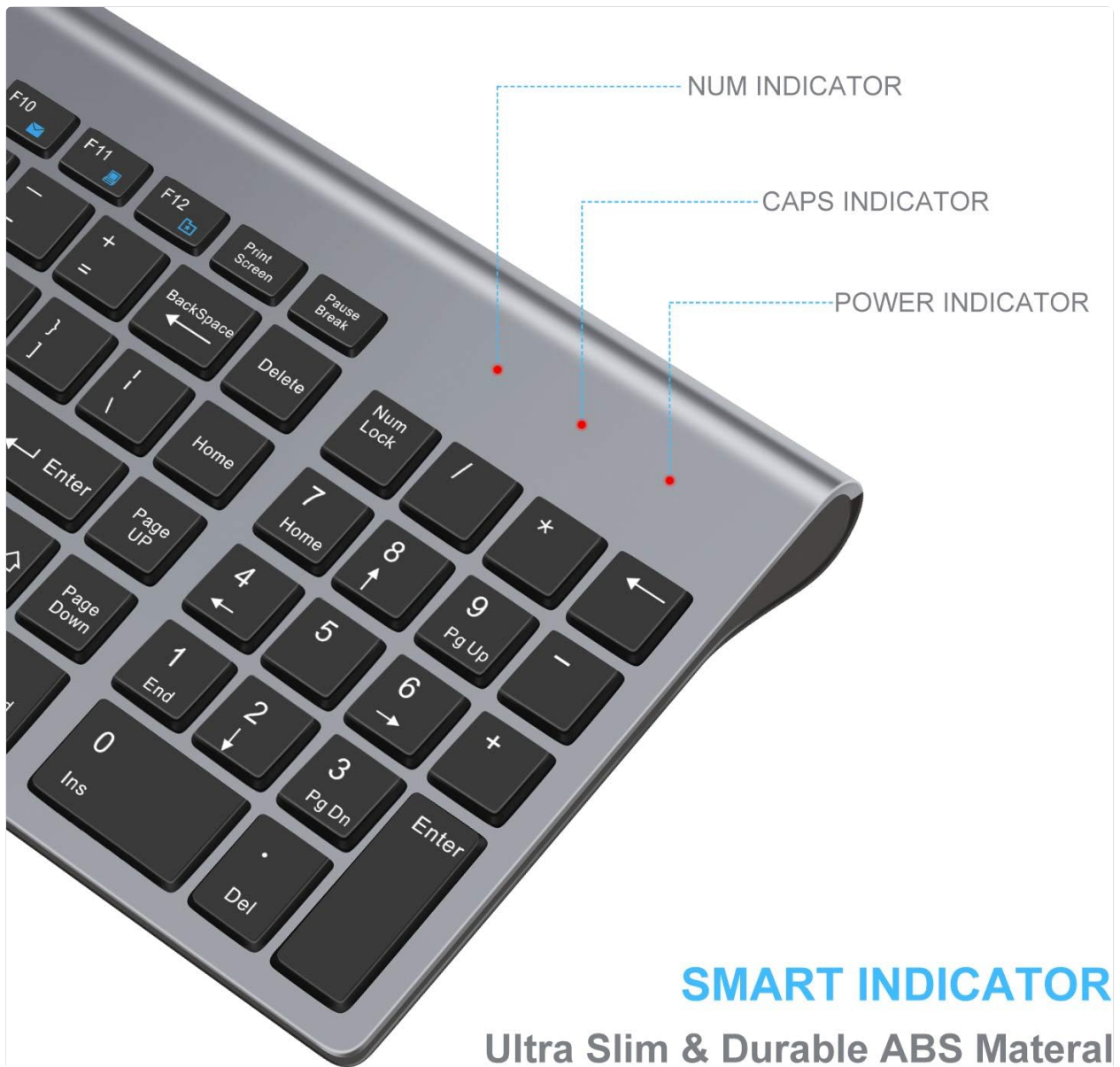
Image 4.3: Close-up of the keyboard's upper right corner, showing the Num, Caps, and Power indicator lights.
