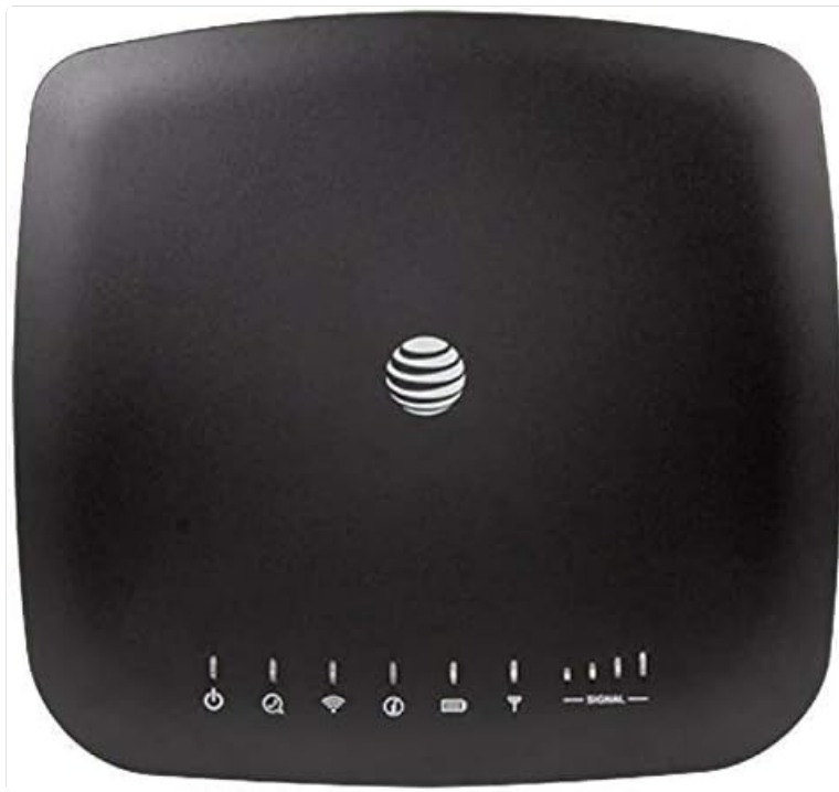
Figure 1: Front view of the Netcomm IFWA 40 Wireless Internet Router, showing the AT&T logo and a row of LED indicators for power, voicemail, Wi-Fi, information, battery, and signal strength.
