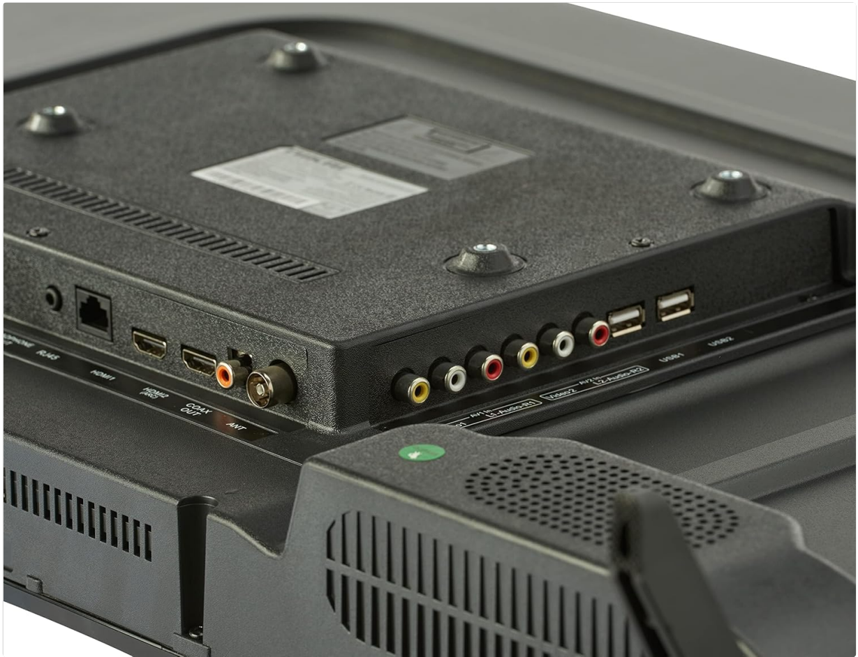
Figure 2: Rear panel connections. Includes 2 HDMI ports, 2 USB ports, VGA, composite video, and audio inputs.
