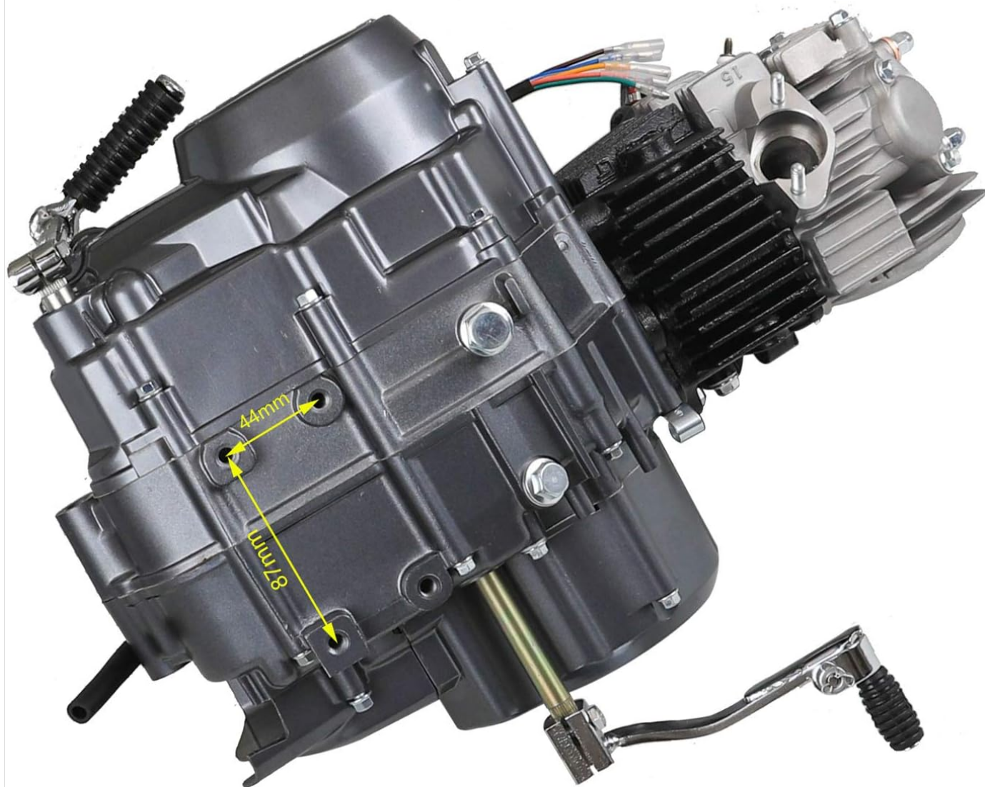
Image: Close-up view of the engine casing highlighting mounting hole dimensions (44mm and 87mm).
