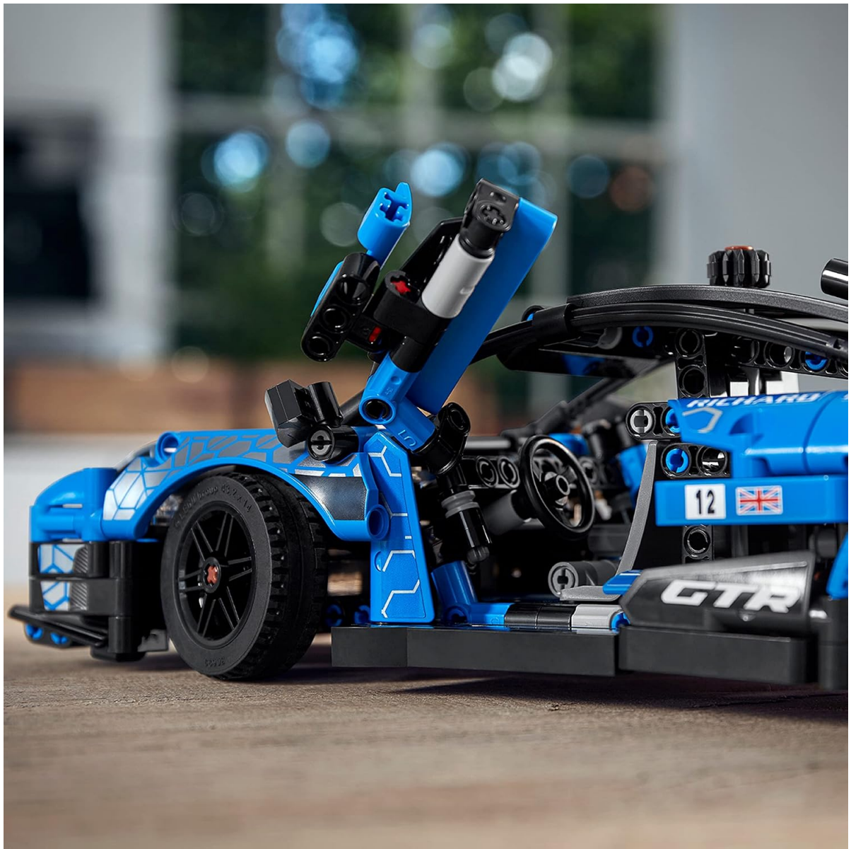
Image 3.2: Detail of the dihedral door mechanism, which opens upwards and outwards.
