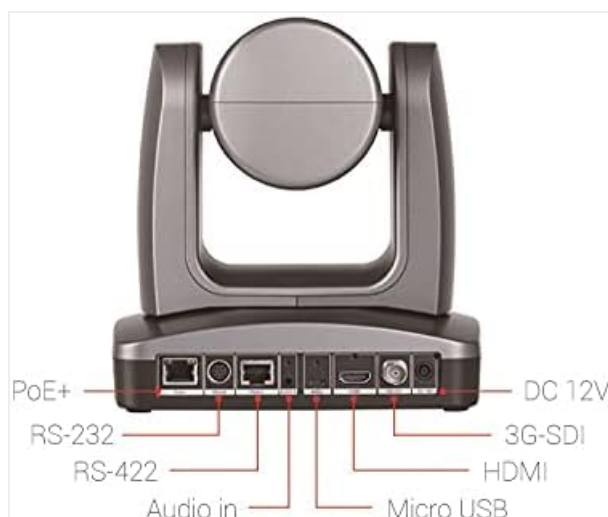
Figure 3.4: Labeled rear panel connections of the AVer PTZ310N camera, indicating PoE+, RS-232, RS-422, Audio In, Micro USB,
