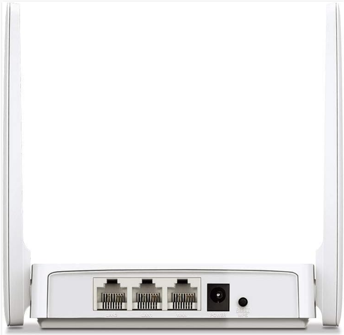
Image: Rear view of the MERCUSYS AC10 router, showing the WAN, LAN, Power, and Reset/WPS ports and buttons.
