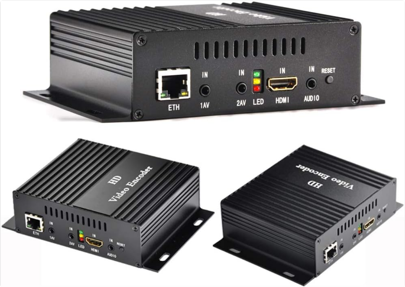
Figure 3.3: Various perspectives of the DMB-8800A encoder, showcasing its compact form factor and heat dissipation design. This provides a comprehensive view of the device's physical attributes.
