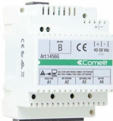
Image: Front view of the Comelit 1456G VIP Gateway Mini SIP. The unit is white with a green and white label indicating 'Art.1456G', 'Comelit', and various port labels such as 'FIXED POE A1', 'VIP SYSTEM A2', 'SETTABLE POE A3', 'NO POE A4'. Power input terminals are labeled '+|-' with a voltage range of '40-56 Vdc'.
