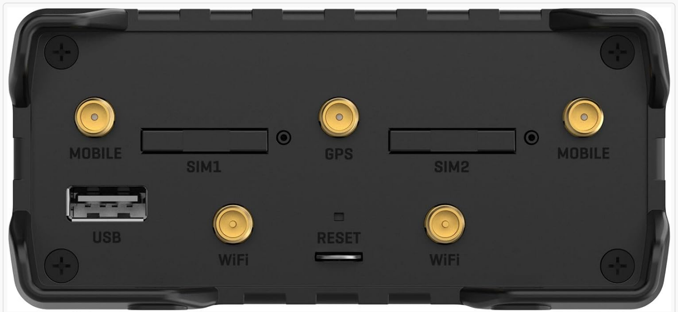
Figure 5.1: Bottom view of the RUT955, highlighting SIM card slots, USB port, GPS antenna connector, Wi-Fi antenna connectors, and the reset button.
