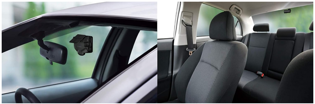
Image: Example of the front camera unit mounted on a vehicle's windshield.
