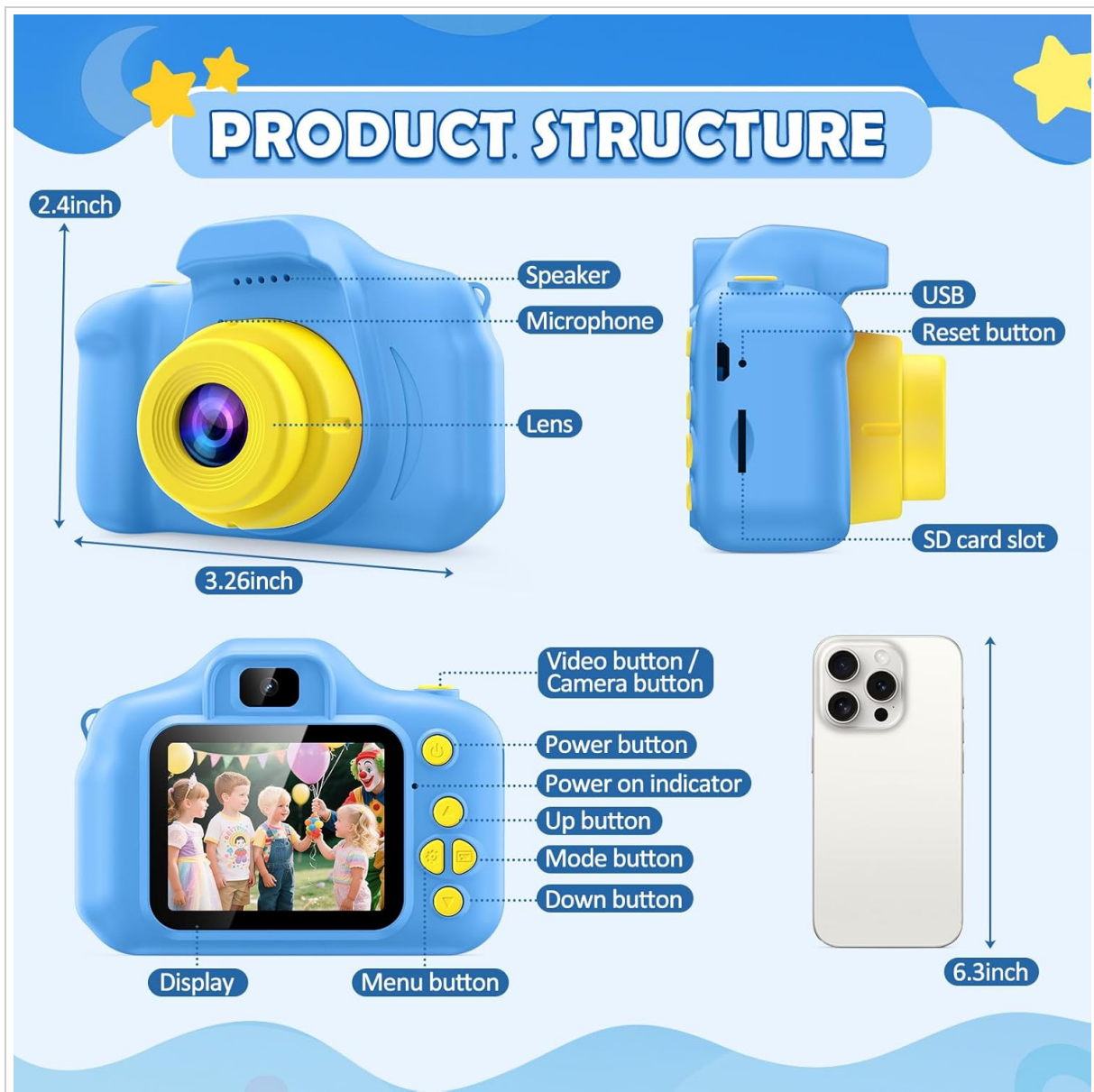
Figure 2: Labeled components of the Desuccus Kids Digital Camera X2.
