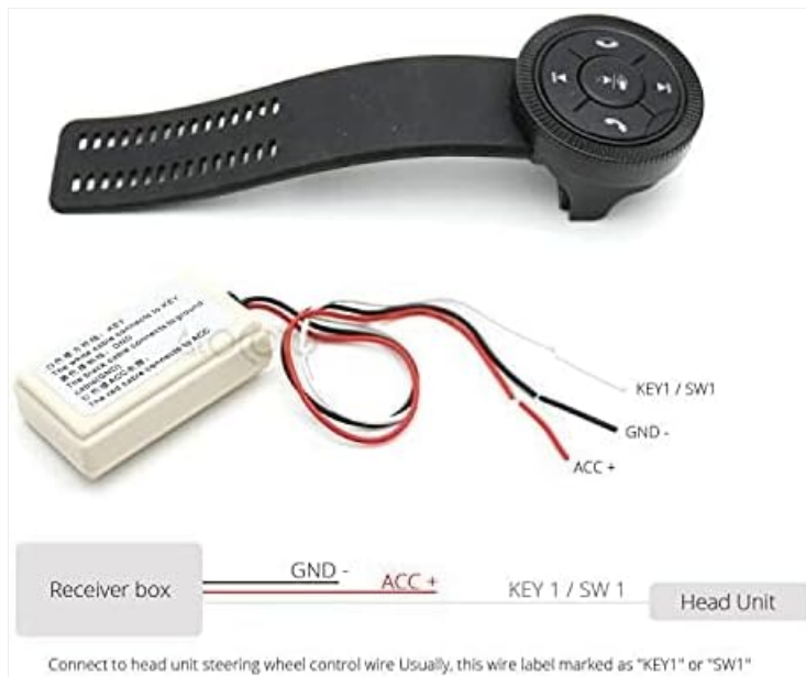
Figure 2: Wiring diagram for the wireless steering wheel control receiver box. This diagram illustrates the connection points for the receiver box. It shows three wires (GND-, ACC+, KEY1/SW1) connecting to the head unit, with the longest wire serving as an antenna.
