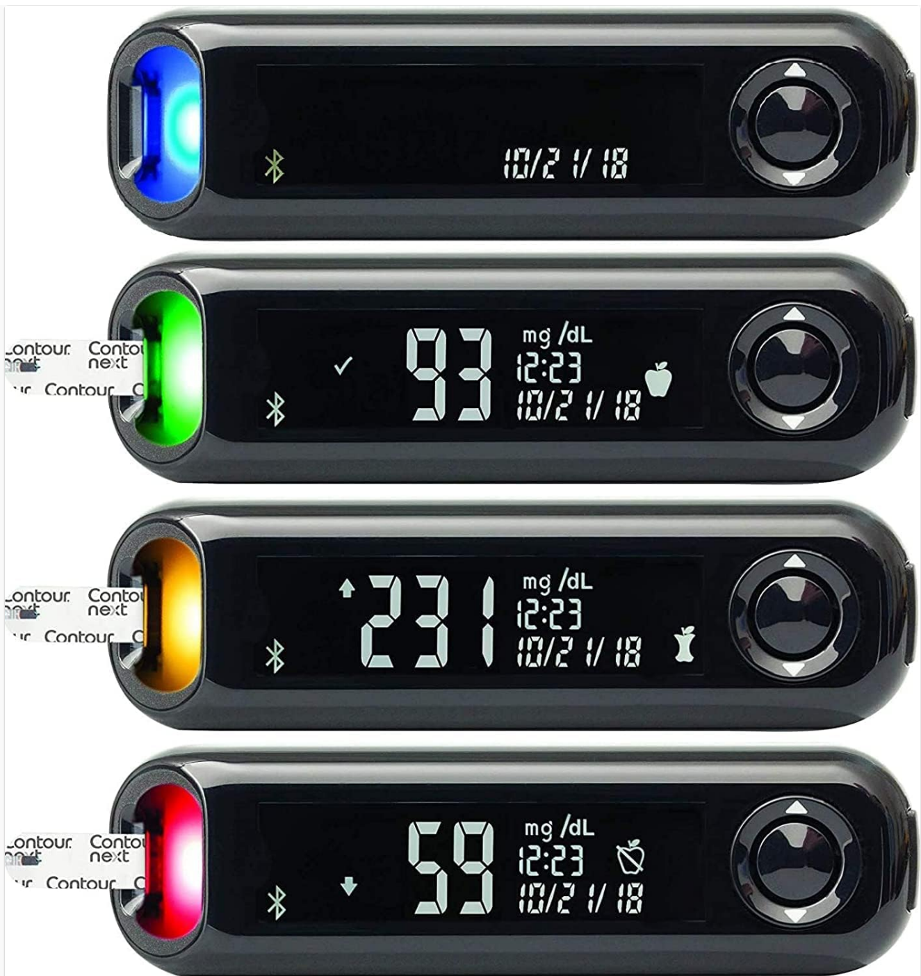
Figure 4.2: Examples of SmartLight indicators on the CONTOUR NEXT ONE meter.
